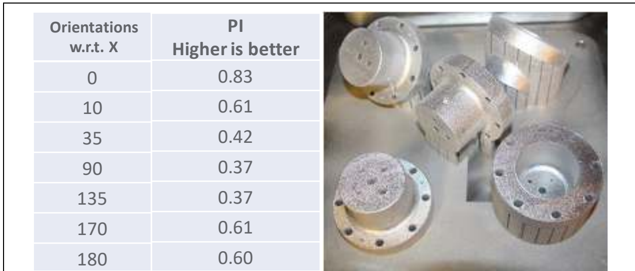
Figure 7. Calculated PI and the printed parts with different orientations
