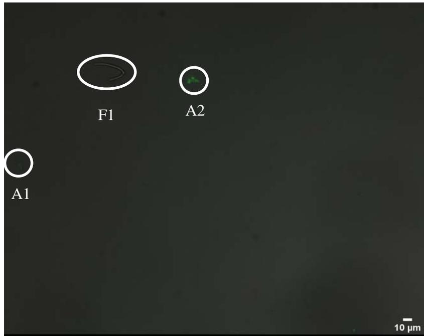
Figure 8. First experiment low concentration FG after introducing MS2. Particle F1 is FG without MS2, and particles A1 and A2 are FG particles with MS2 collocated.
