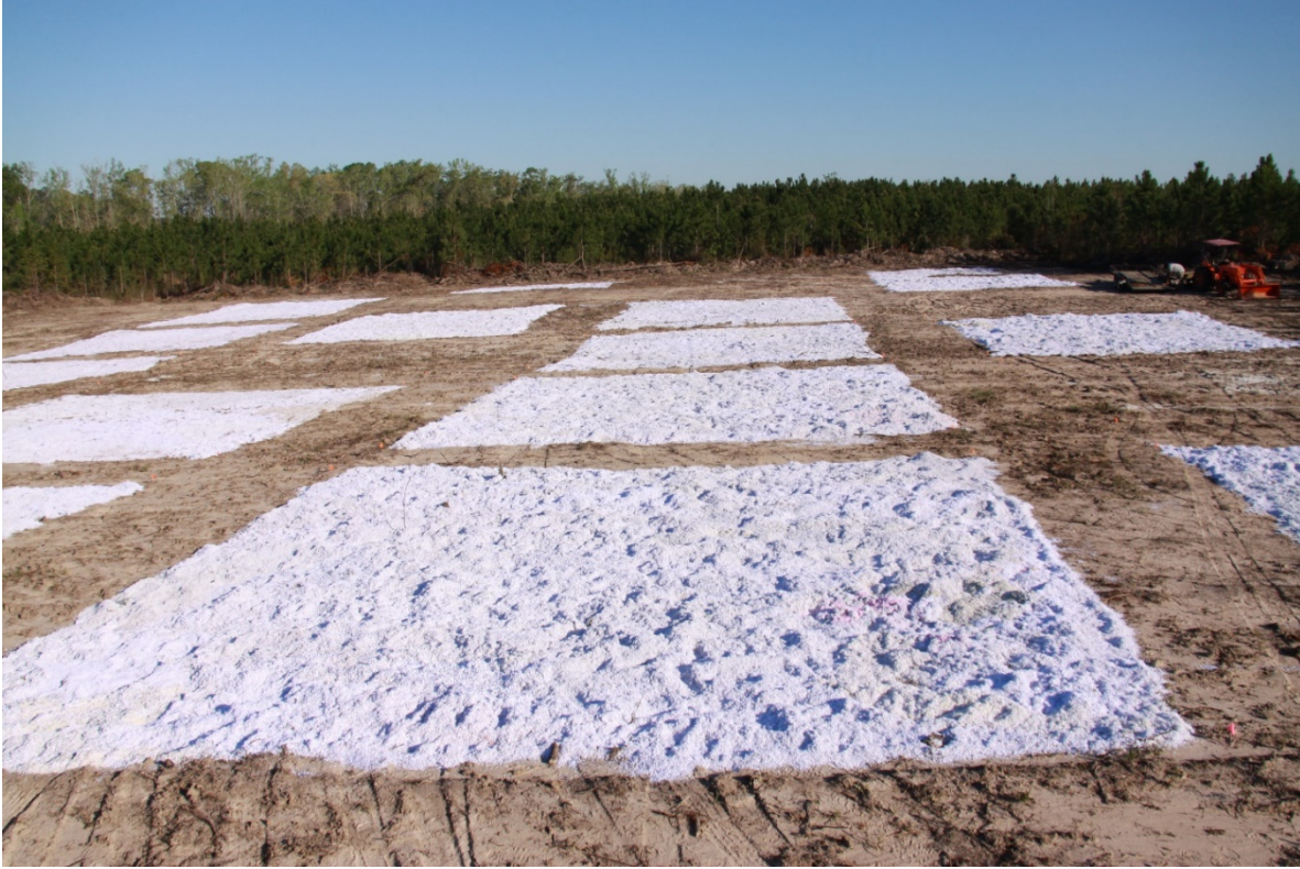
Figure 8. Paper is spread evenly over plots. Plots contained varying application rates.
