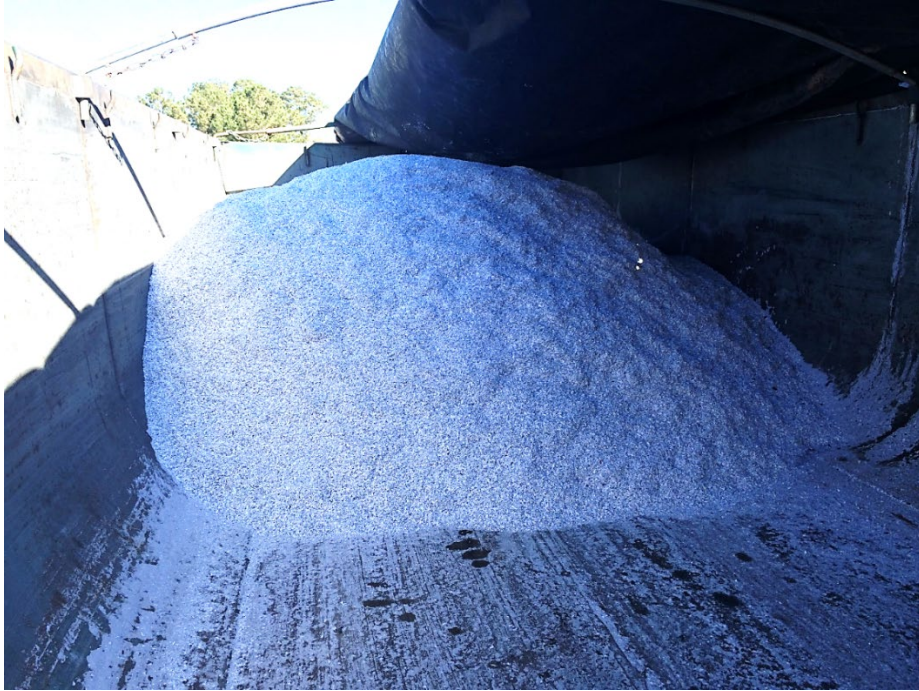
Figure 2. Approximately 1 ton of pulverized paper in a rented 20 cubic yard rolloff container.
