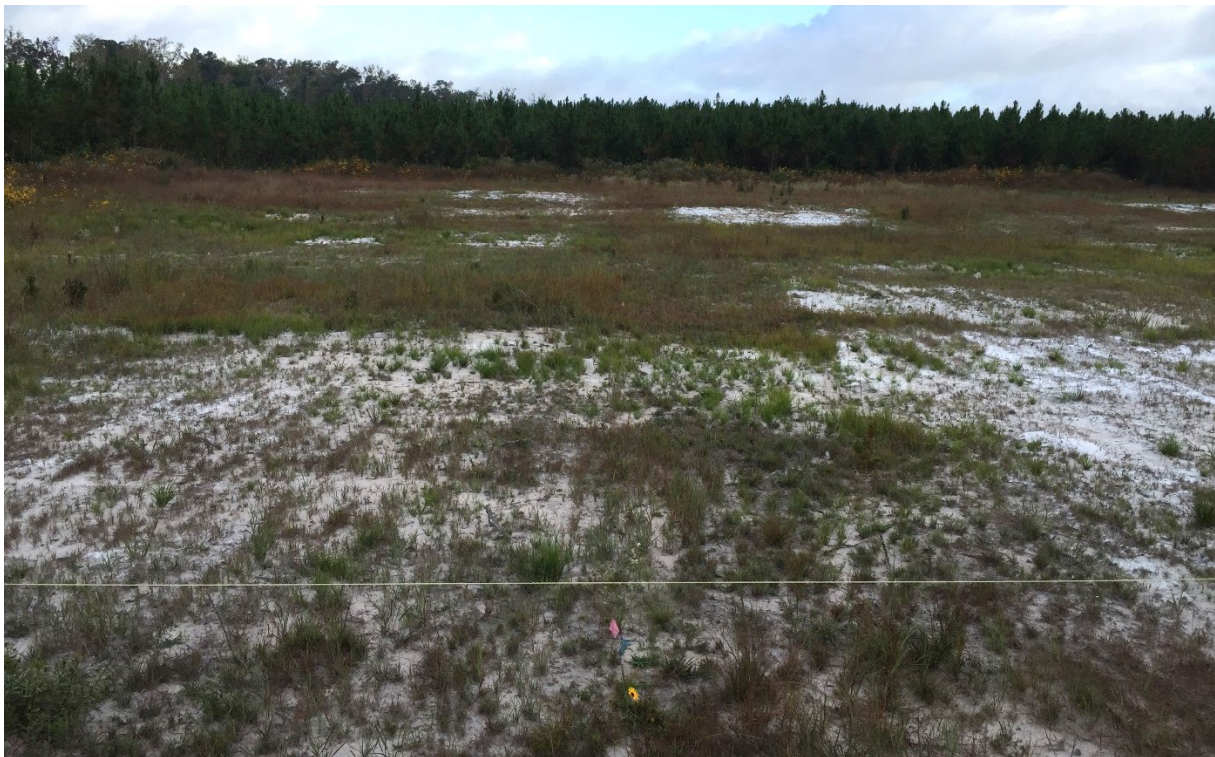
Figure 13. Paper application after 1 growing season. The paper is still visible in 24 and 32 tons per acre application rates. Areas where paper is not visible received paper application rates of 16 tons per acre or less.
