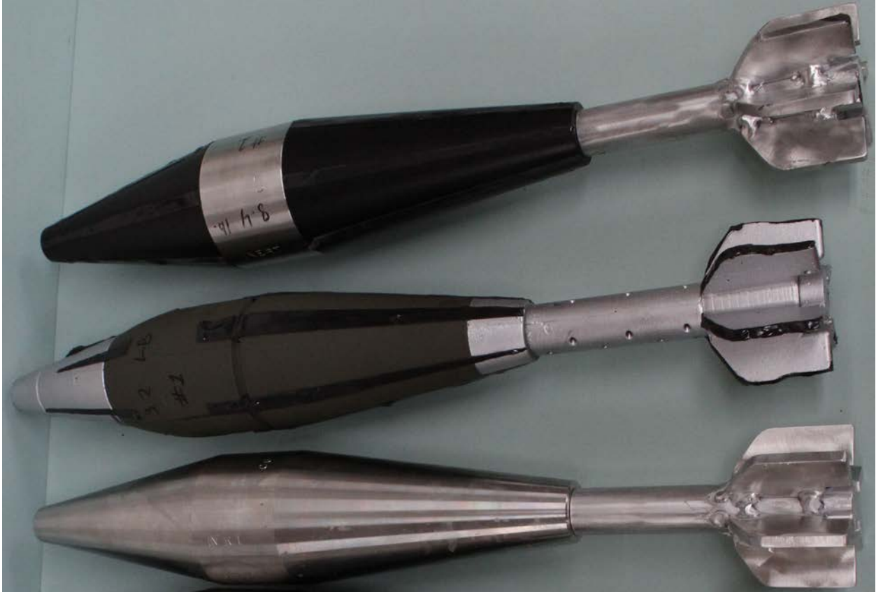
Figure 4. Photo of the surrogate (top), purchased replica (middle), and the replica fabricated with a solid stainless steel body and aluminum tail section (bottom) for the 81 mm mortar type.
