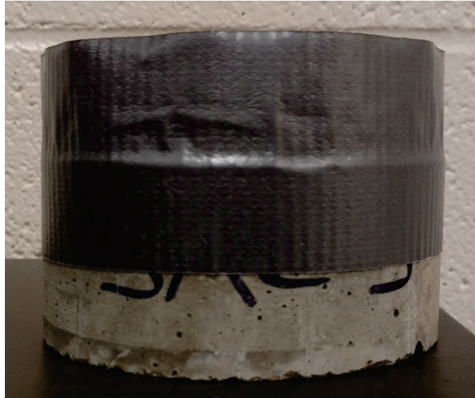
Figure 20. Puck with tape reservoir.
