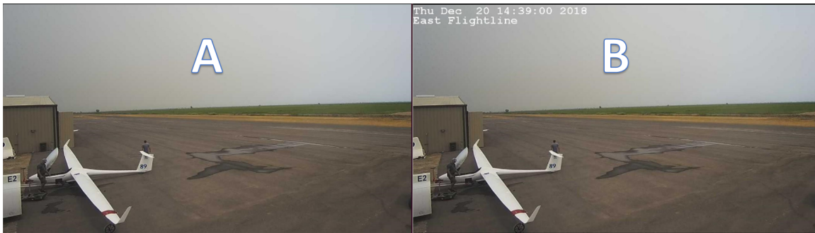
Figure 22. The Python script has the capability to draw date and time on the camera image
