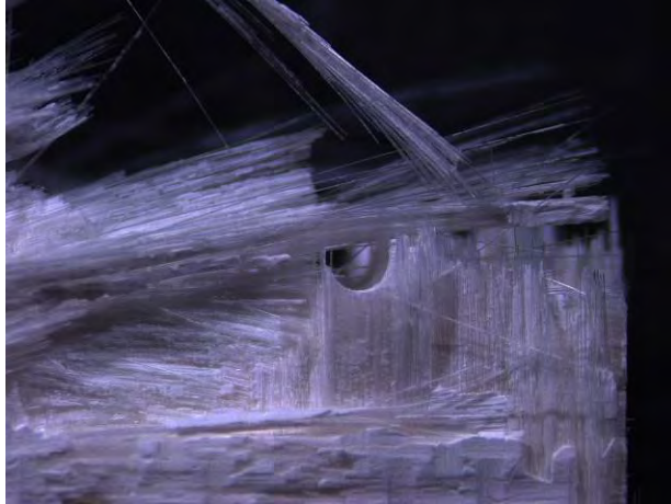
Figure A. 8: Fracture surface of specimen #3, tested in tension to failure at 1200°C in air
