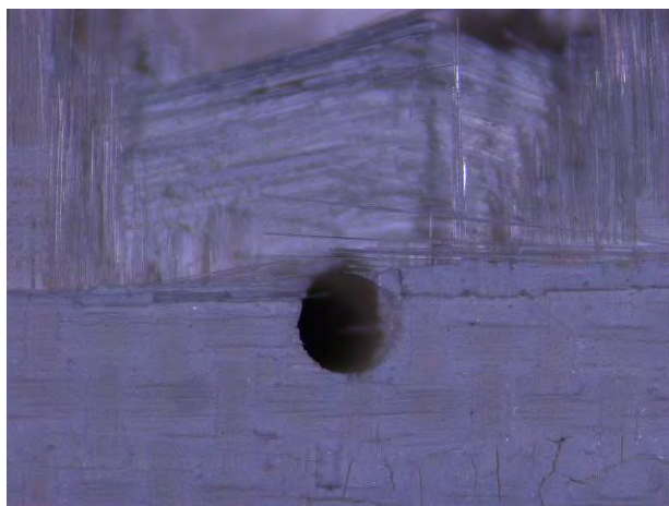
Figure A. 34: Fracture surface of specimen #8, tested in creep at 1200°C in air ( \sigma_{cr} = 150 MPa, t_f = 0.01 h)
