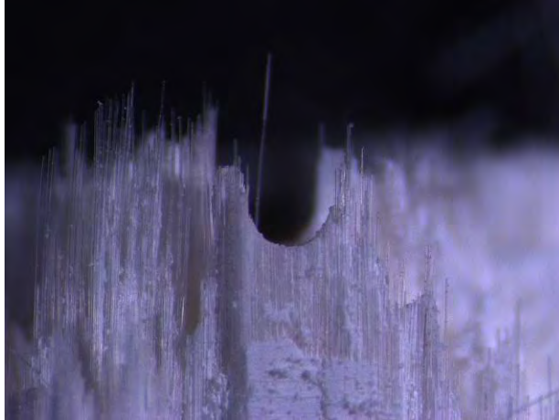
Figure A. 62: Fracture surface of specimen #11, tested in creep at 1200°C in steam ( \sigma_{cr} = 150 MPa, t_f = 0.04 h)
