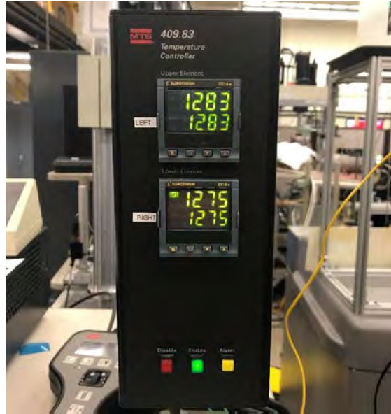
Figure 10: MTS Temperature Controllers
