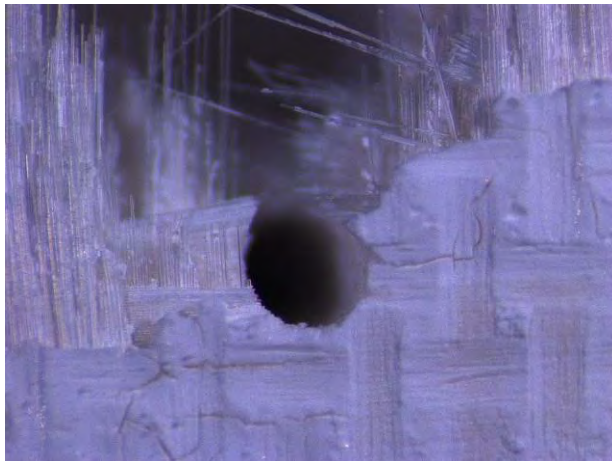
Figure A. 63: Fracture surface of specimen #11, tested in creep at 1200°C in steam ( \sigma_{cr} = 150 MPa, t_f = 0.04 h)
