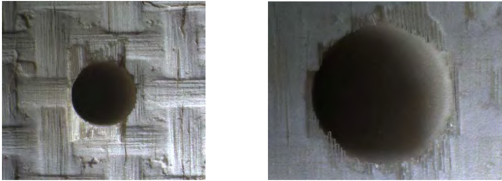
Figure 37: Pre-test optical micrographs of N720/A specimens with diamond-drilled holes showing material in the vicinity of randomly selected holes
