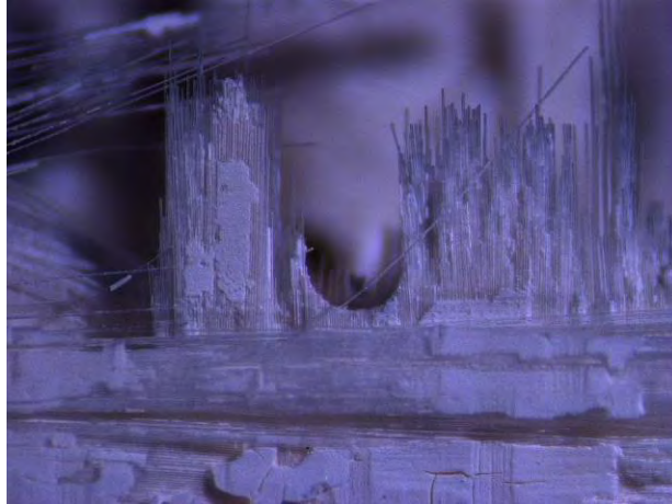
Figure A. 5: Fracture surface of specimen #3, tested in tension to failure at 1200°C in air
