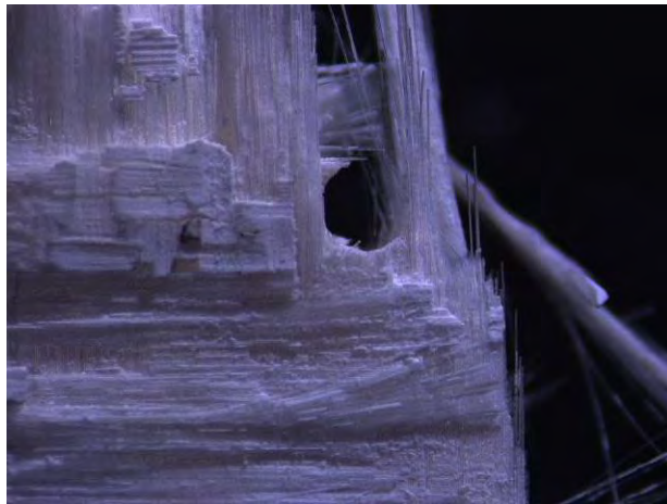
Figure A. 7: Fracture surface of specimen #3, tested in tension to failure at 1200°C in air
