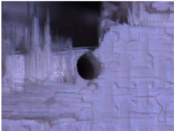
Figure A. 42: Fracture surface of specimen #12, tested in tension to failure following 100 h creep at 46 MPa at 1200°C in steam
