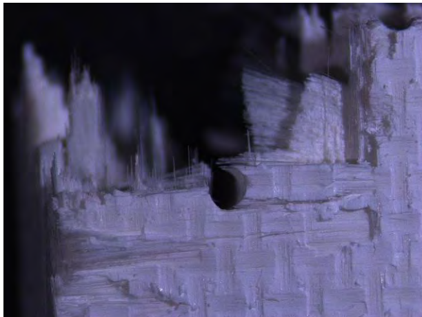
Figure A. 41: Fracture surface of specimen #12, tested in tension to failure following 100 h creep at 46 MPa at 1200°C in steam
