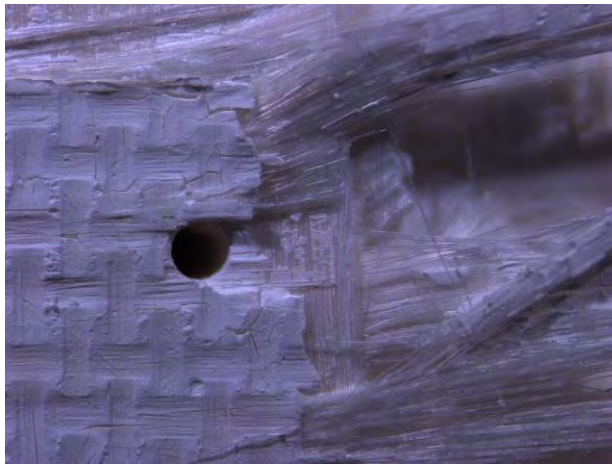
Figure A. 10: Fracture surface of specimen #3, tested in tension to failure at 1200°C in air
