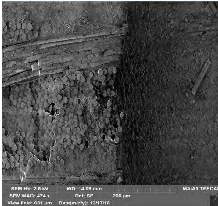
Figure 52: Fracture surface of an N720/A specimen with diamond-drilled holes tested in creep at 1200°C in steam ( \sigma_{cr} = 93 MPa, t_f = 6.05 h)
