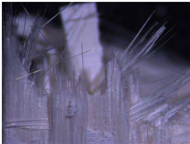
Figure A. 60: Fracture surface of specimen #11, tested in creep at 1200°C in steam ( \sigma_{cr} = 150 MPa, t_f = 0.04 h)
