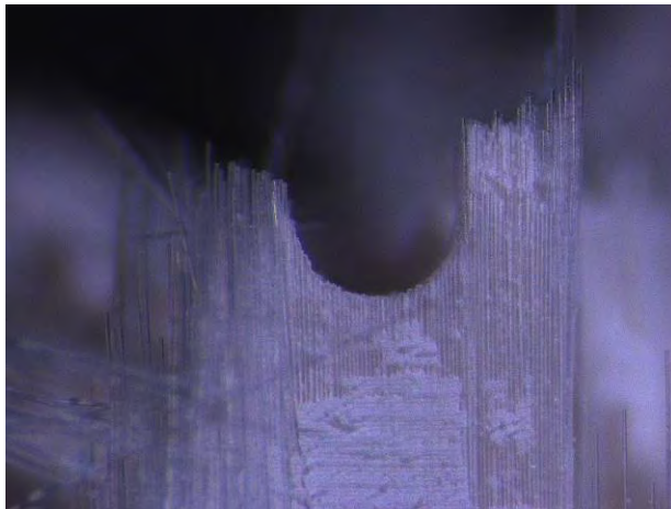
Figure A. 53: Fracture surface of specimen #9, tested in creep at 1200°C in steam ( \sigma_{cr} = 116 MPa, t_f = 0.61 h)
