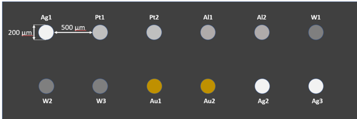
Figure 22. Diagram of shadow mask contact layout on UO_2 .
