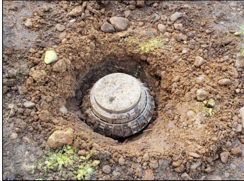
Figure 139: VS2.2 mine surrogate being buried at 1”.
