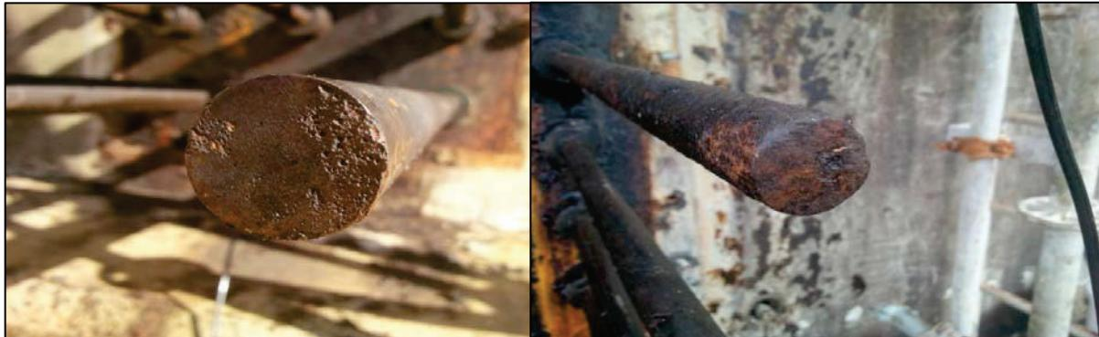
Figure 4. Pitted rod and surface corrosion on rod.
