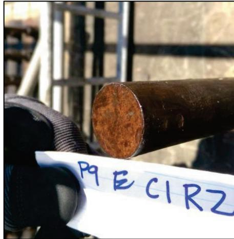
Figure 5. Typical rod without corrosion.
