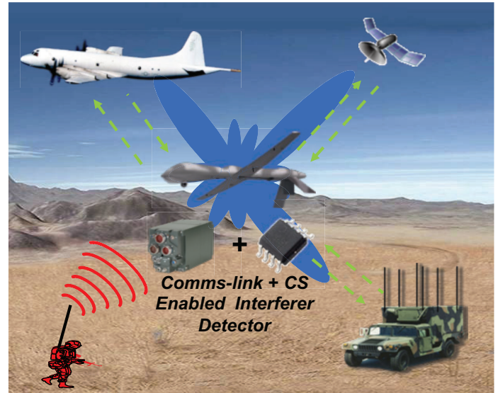
Fig. 1: An example of how a CS-assisted interferer detector creates local EM environmental awareness and helps a UAS comms-link by avoiding adversarial jamming.
