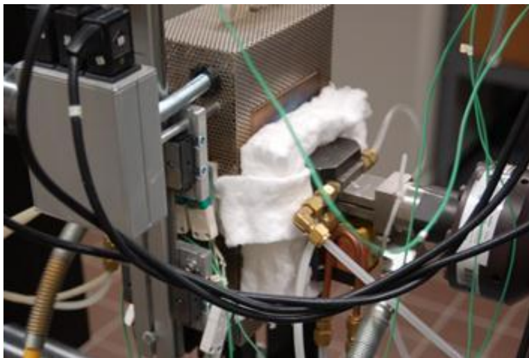
Figure 25. Photograph of Furnace Packed with Custom-Cut Insulation
