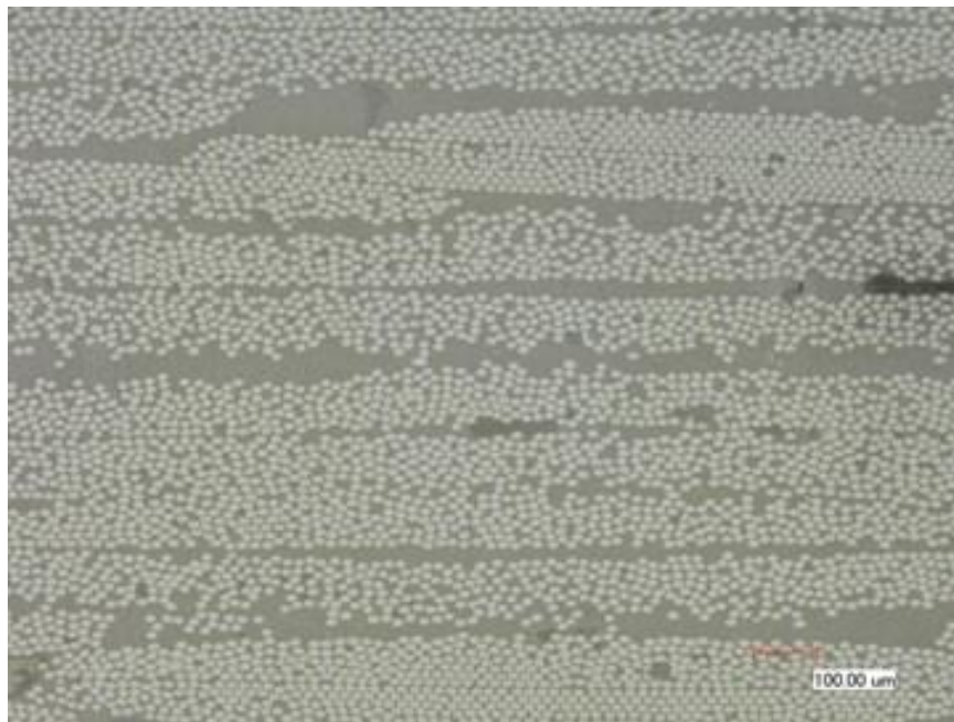
Figure 12. Representative \pm 45 Micrograph of N720/AS Microstructure (200 \times , C)
