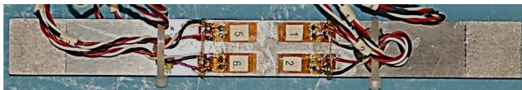
Figure 18. Straight-Sided Steel Bar Alignment Specimen with Eight Strain Gages
