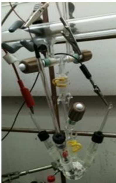
Figure 1. Picture of electrochemical cell set-up attached to the vacuum line. The cell consists of four necks, one for each electrode and one for connecting the cell to the vacuum line. Wires connecting the electrodes to the external circuit are sealed with leaded glass.
