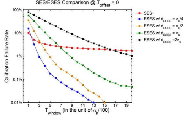
Figure 2 SES/ESES calibration failure rate vs. calibration target window when  $T_{\text{offset}} = 0$ .
