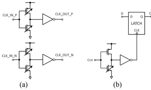
**Figure 8 Conceptual circuits for high resolution phase/delay calibration applications: (a) differential signals calibration; (b) delay calibration of synchronous signals.**
