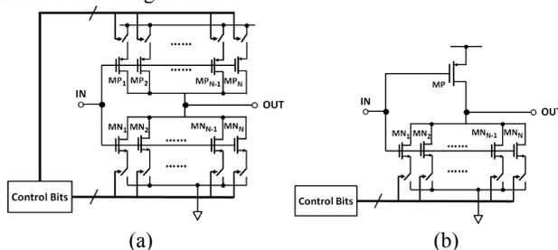
**Figure 7 ESES-based phase/delay calibration conceptual circuit: (a) tunable rising and falling edge; (b) tunable falling edge only.**
