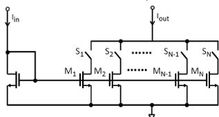
**Figure 6 ESES-based current calibration conceptual circuit.**
