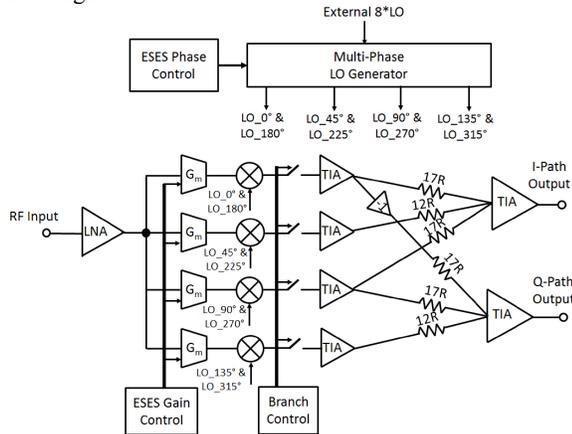
**Figure 9 Harmonic rejection receiver architecture with ESES-based calibration.**
