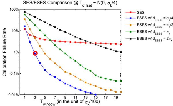
**Figure 3 SES/ESES calibration failure rate vs. calibration target window when  $T_{\text{offset}} \sim N(0, \sigma_k/4)$ .**
