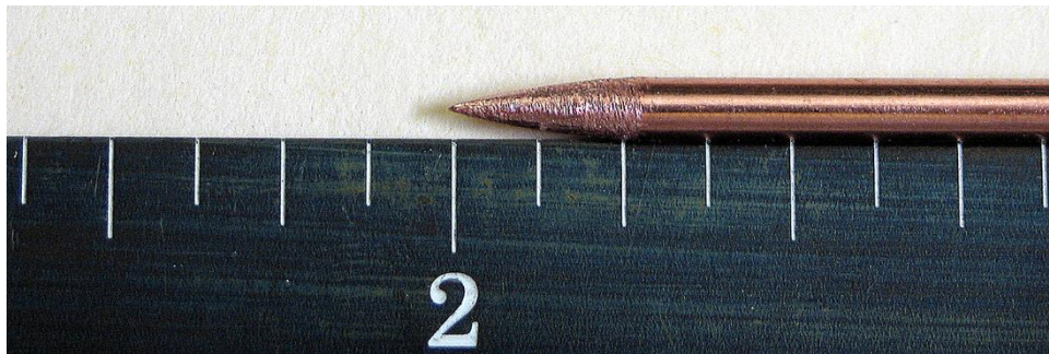
Fig. A-6 A hand-ground L/D = 2.7 anode point (scale is in inches, 1 inch = 25.4 mm)
