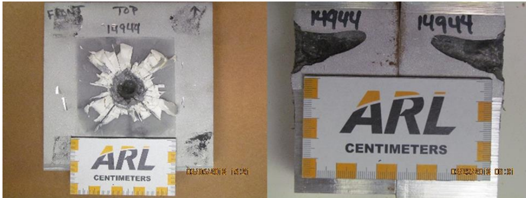
Fig. 17 PSD alumina tiles after impact
