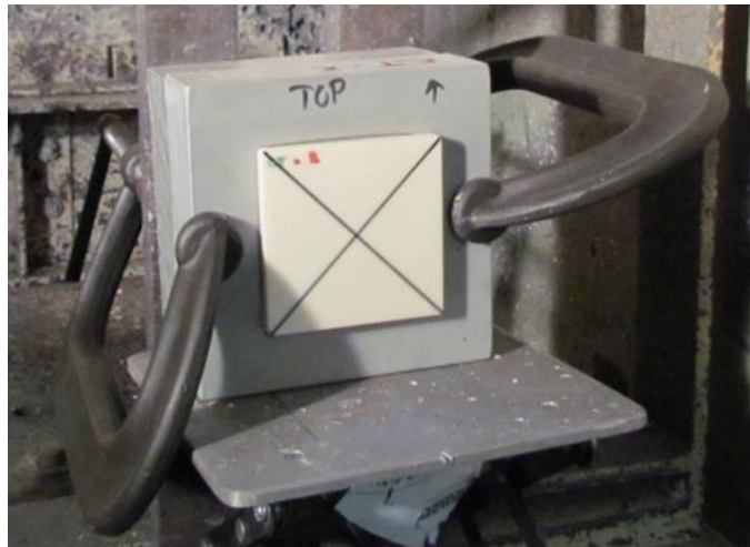
Fig. 5 Initial conditions of ceramic composite samples in fixture
