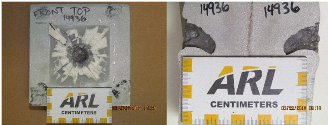
Fig. 18 DIW alumina tiles after impact
