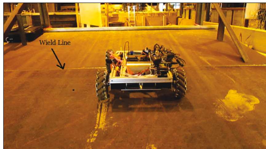
Figure 56. Prototype Mobile Sensor Inspection Platform inspecting steel plate.
