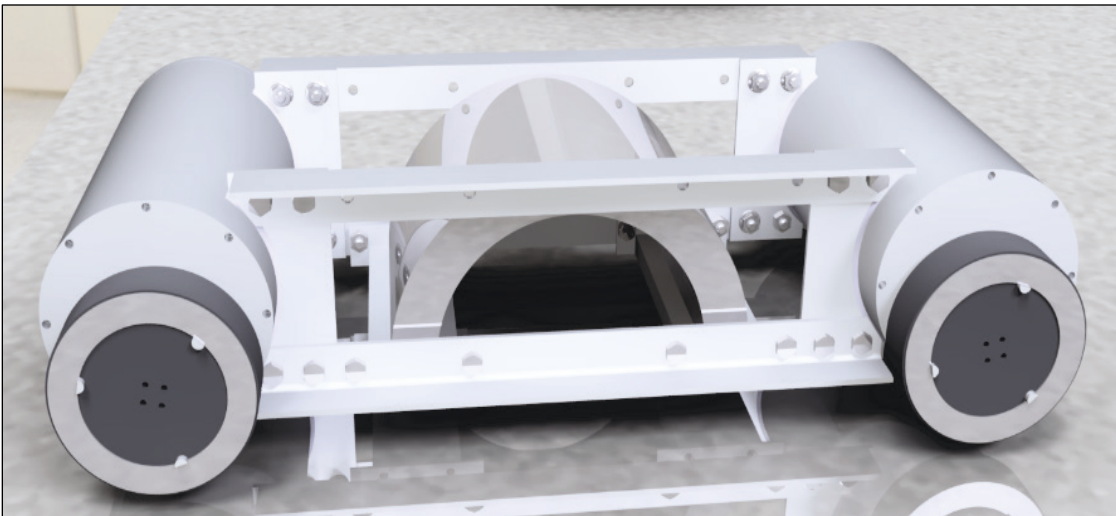
Figure 47. Present MFL magnetic crawler test platform capable of being submerged, showing the waterproof housing around the motors (dimensions: 14 in. wide, 22 in. long, and 8 in. tall).
