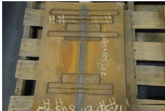
**Figure 6: Phase 1 I-plate Marked Samples for Standardized Weld Characterization Tests**
