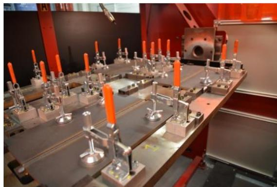
**Figure 1: Fixture for Robotic Welding of Phase 1 plate**
