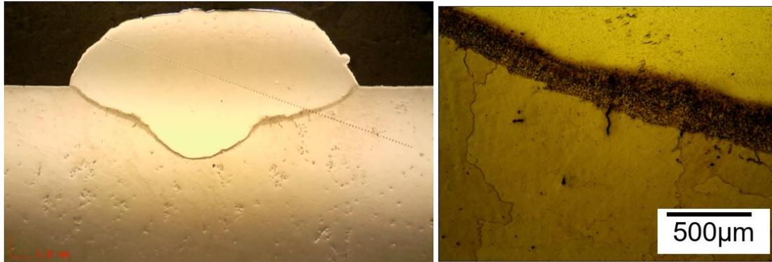
**Figure 1. (Left) Metallographic cross section of 308L weld bead on cast FeMnAl steel plate showing a number of casting defects as well as (right) micro cracks forming at the grain boundary at the unmixed zone**
