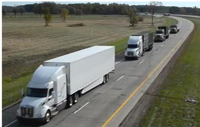
Figure 1. Auburn CACC system on Highway I69 with four vehicle platoon.
