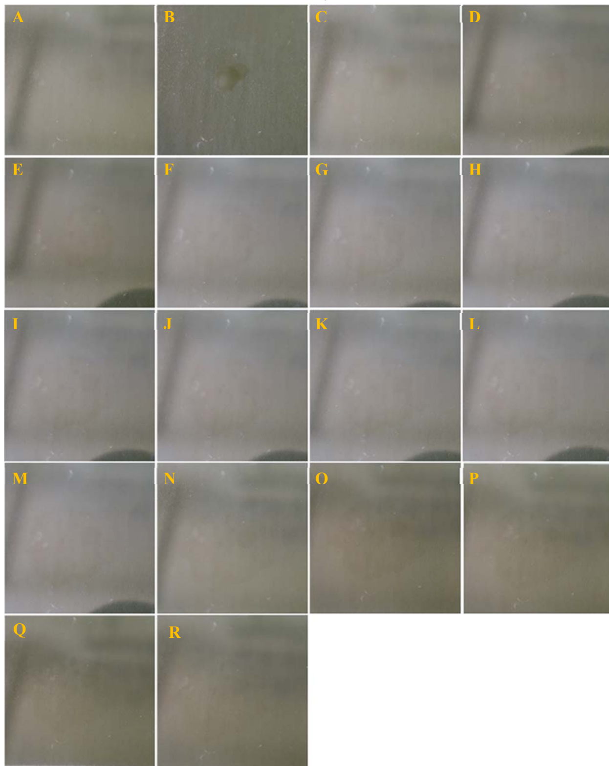
Fig. B1 — DFP on Fomblin Y oiled paint. Images of a coupon before application (A) and at 0 (B), 0.5 (C), 1 (D), 1.5 (E), 2 (F), 2.5 (G), 3 (H), 3.5 (I), 4 (J), 4.5 (K), 5 (L), 5.5 (M), 10 (N), 15 (O), 20 (P), 25 (Q), and 30 (R) min following application of the target. These images were collected with a glass cover in place to limit evaporation. Reflections from the cover can be seen in some images.
