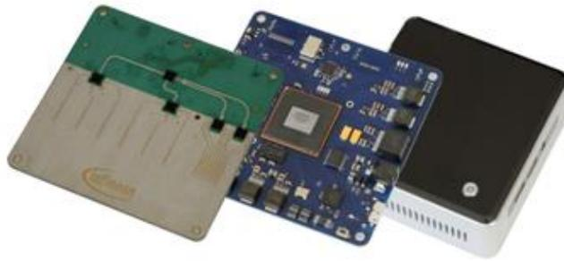
Fig. 1 - Inras modular radar test bed.
