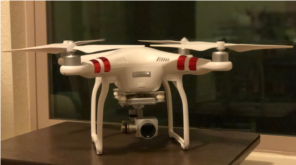
Figure 1. Image of the DJI Phantom 3 Standard. Digital camera with 3D gimbal shown below the UAS.
