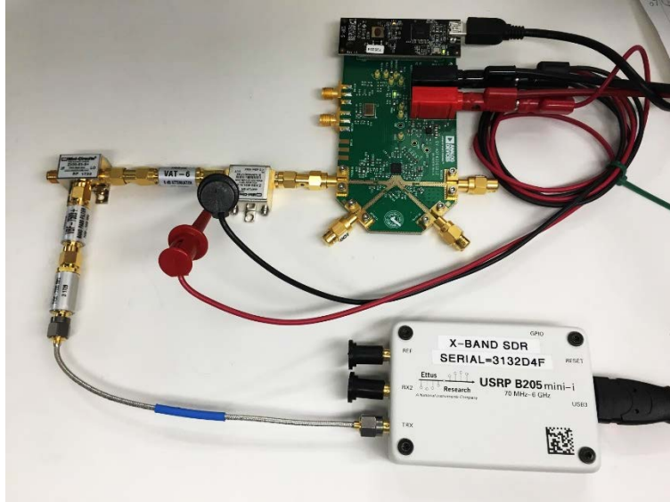
Figure 64. X-band Conversion Circuitry.
