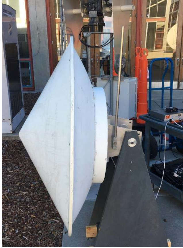
Figure 34. Photo of C-Band Dish Antenna.
