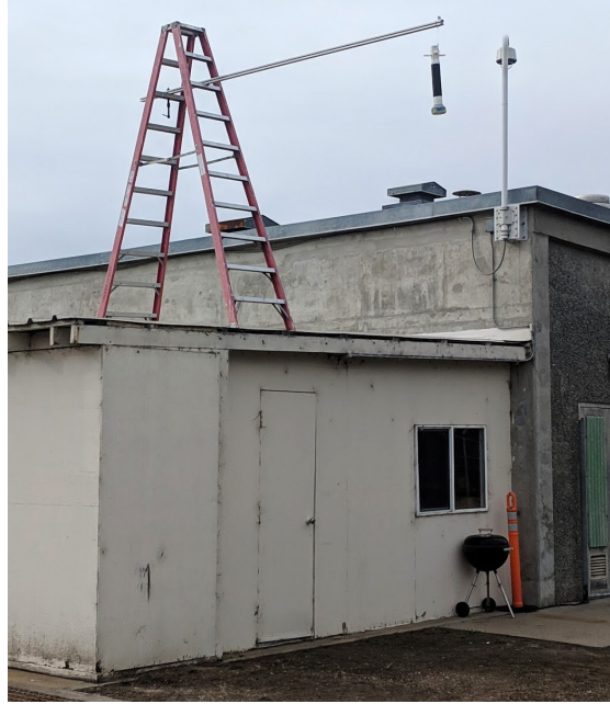
Figure 19. Nose-down deployment test configuration.
