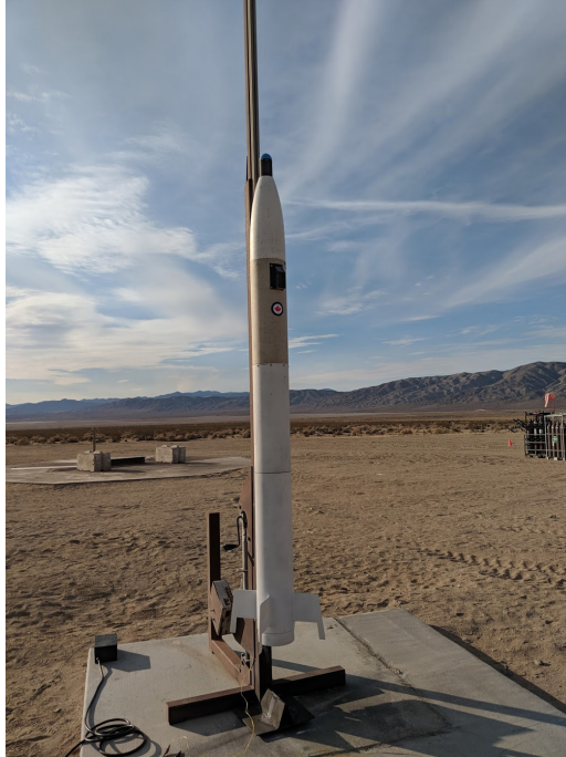
Figure 25. Nose-mounted submunition on rocket in launch configuration.
