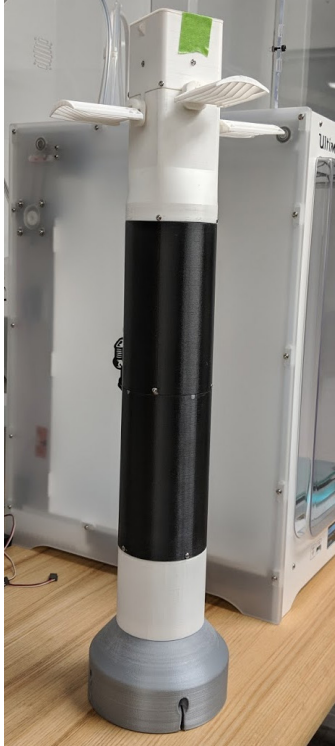
Figure 17. Second kill mechanism design fitted with drop test rig
