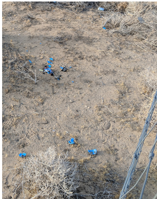
Figure 29. Bomblet front half debris field at impact location.
