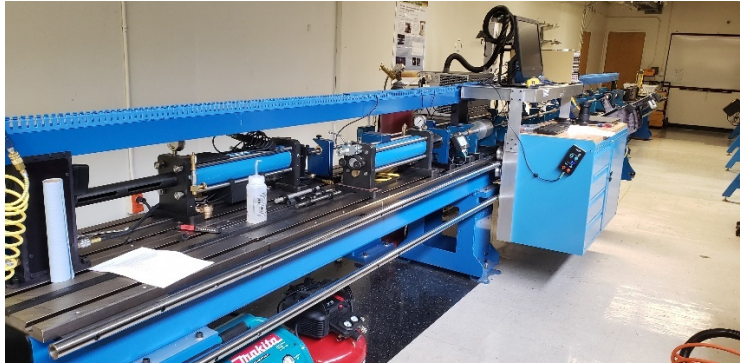
Figure 10. NPS Split Hopkinson pressure bar
