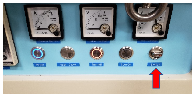
Figure 10: Front console of furnace. Switch.
