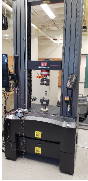
Figure 11. NPS Instron 5982 used for quasi-static testing
