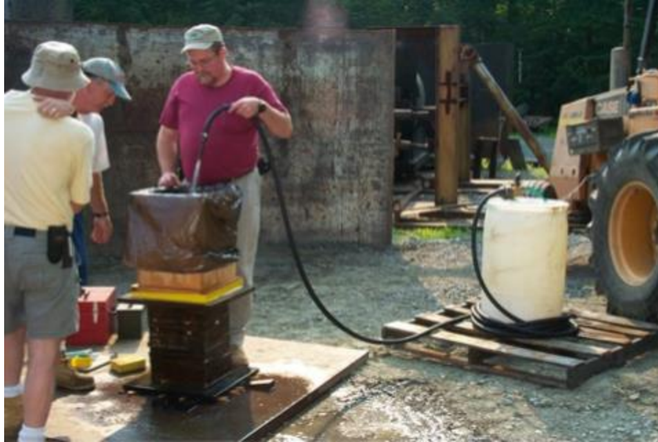
Fig. 2 Filling target with 500 mm of water
