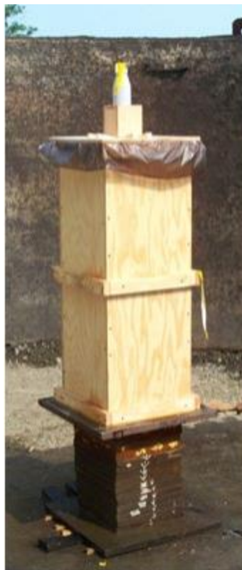
Fig. 3 Typical experimental setup. Target with 1000 mm of water is shown. The wooden target assembly has a hole cut in the top so the first material impacted by the shaped charge jet is water.
