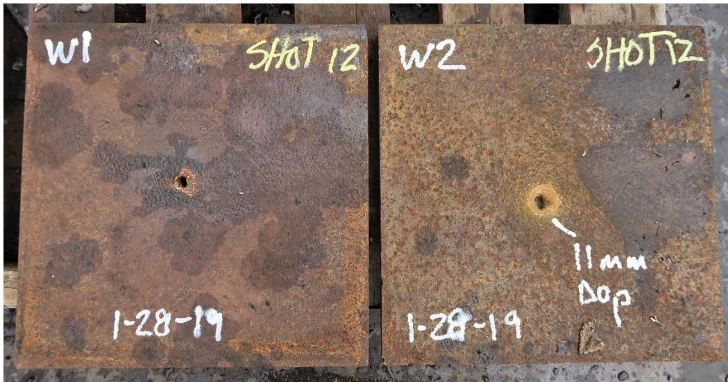
Fig. 8 Typical postexperimental debris. Witness plates from 1090-mm ice target are shown. The jet stopped in witness Plate 2 (W2).
