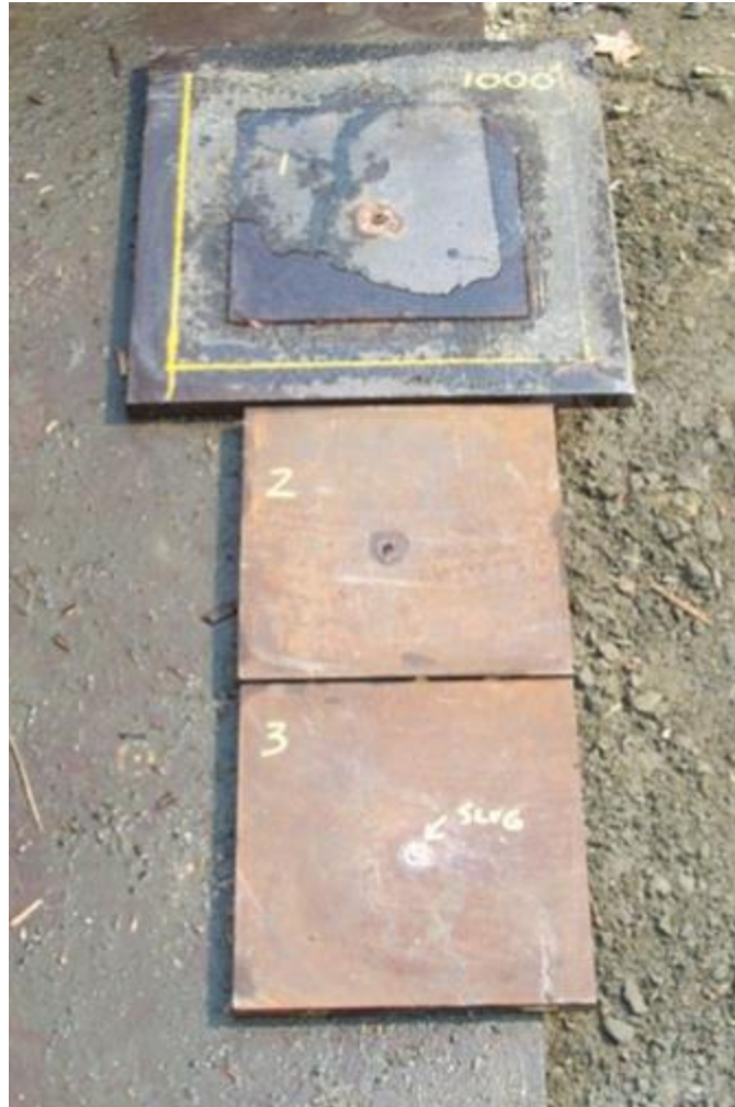
Fig. 4 Typical postexperimental debris. Debris from target with 1000 mm of water is shown. The jet stopped in witness Plate 3.
