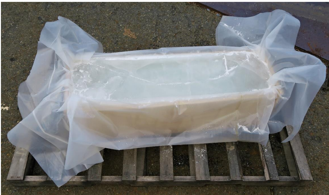
Fig. 7 Typical box used to hold and freeze the water. The 1090-mm box is shown.
