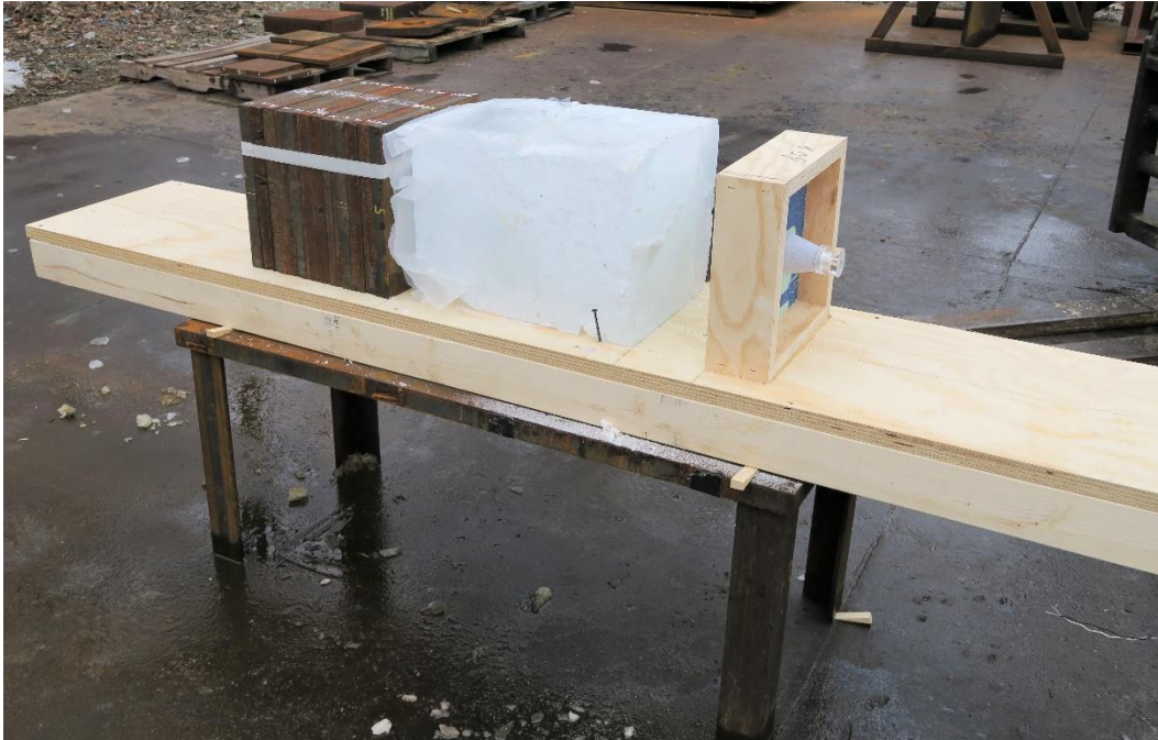
Fig. 6 Typical experimental setup showing a 545-mm ice target
