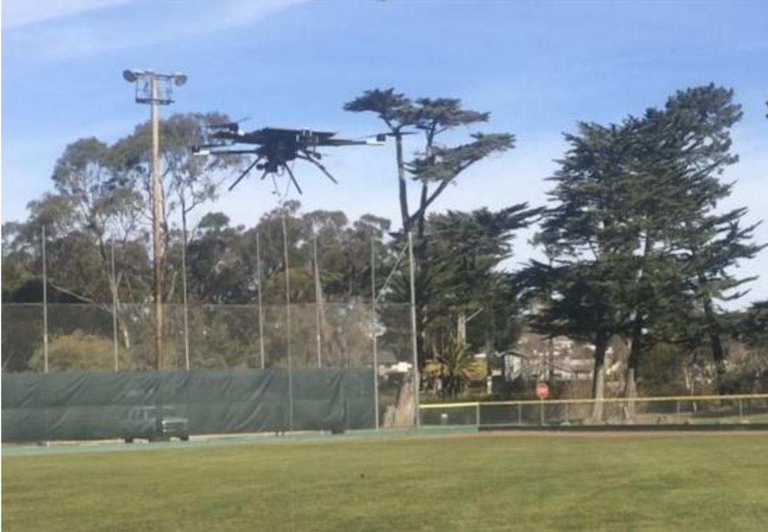
Figure 30. Condor Outdoor Flight Testing in its Fully Assembled Configuration
