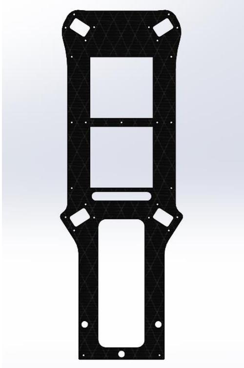
Figure 18. Condor Lower Frame Design with Battery Cutouts
