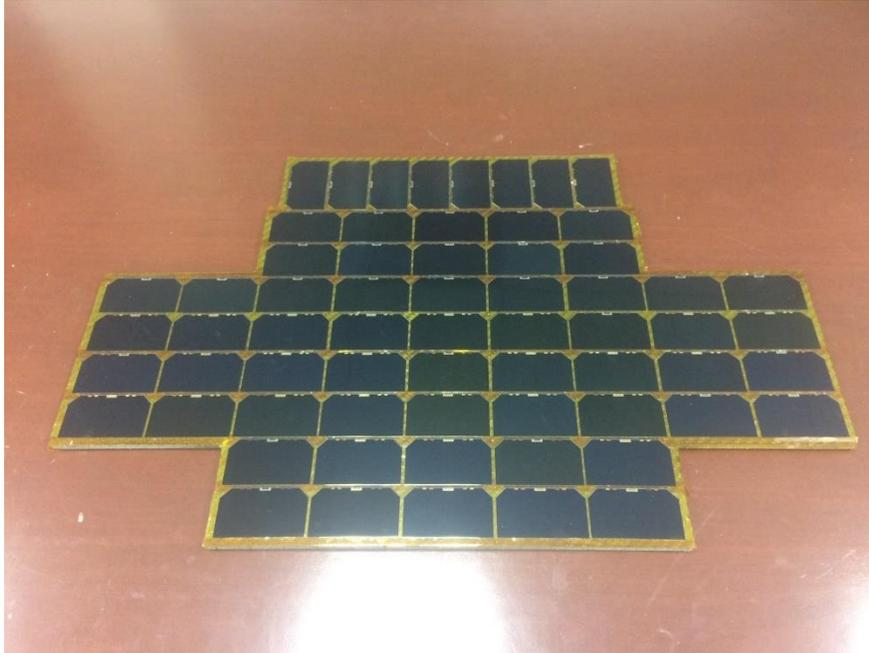
Figure 16. 64 Solar Cells Hand-Mounted on the Condor PV Array
