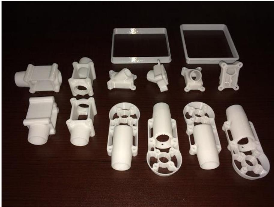
Figure 21. Condor Parts Designed in Solidworks and 3D Printed
