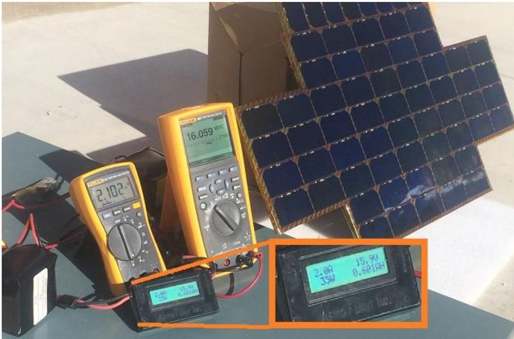
Figure 24. PV Array and MPPT Power Output Test Setup
