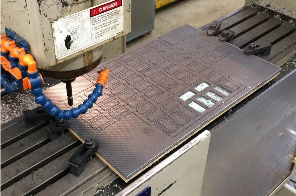
Figure 14. Condor PV Array Being Cut on a CNC Machine
