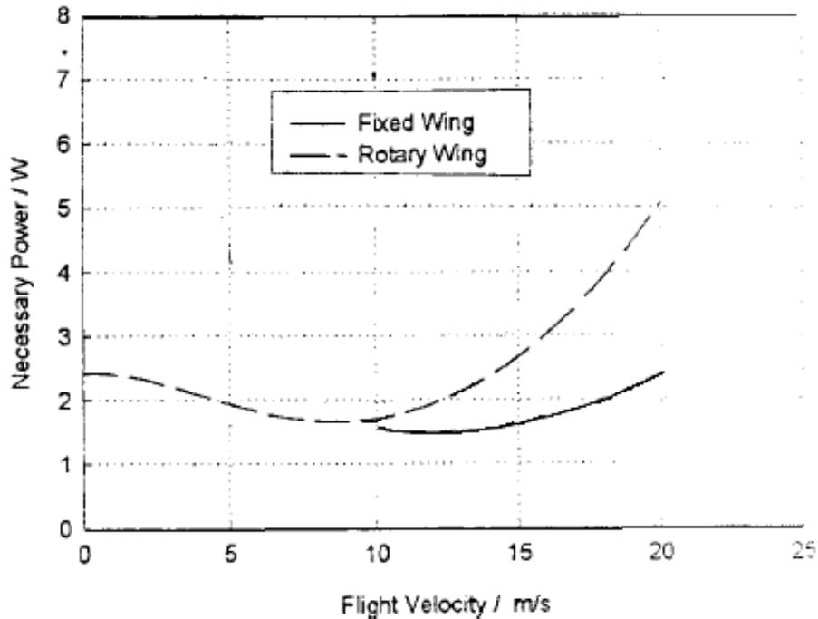
Figure 2. Comparison of Power Efficiency in Fixed and Rotary Wing Aircraft. Adapted from [8].
