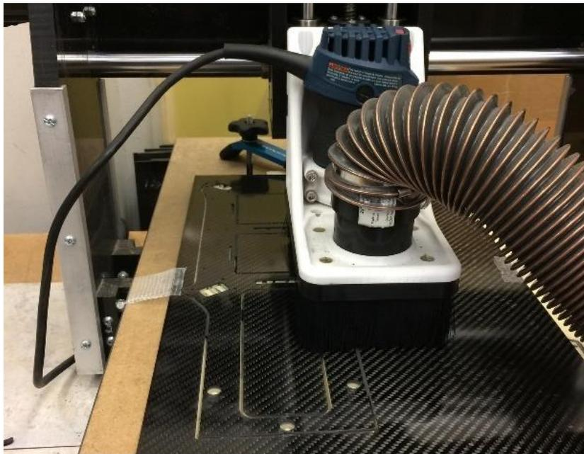
Figure 20. Condor Lower Frame Being Cut on CNC Router
