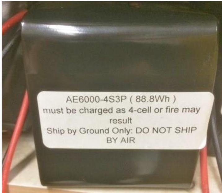
Figure 9. Li-Po 4S3P Batteries Used on Condor
