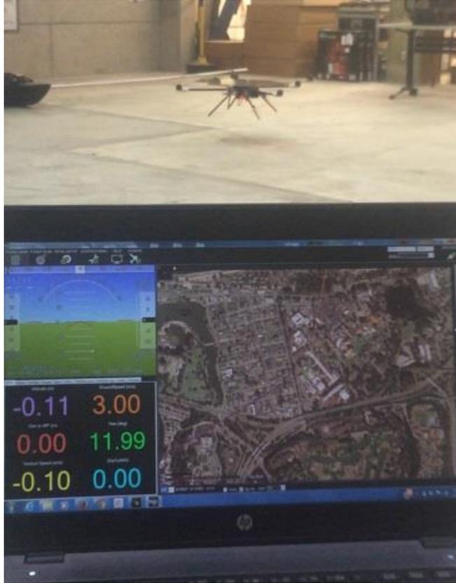
Figure 29. Condor Fully Assembled Stable Flight Indoors Mission Planner GUI in View
