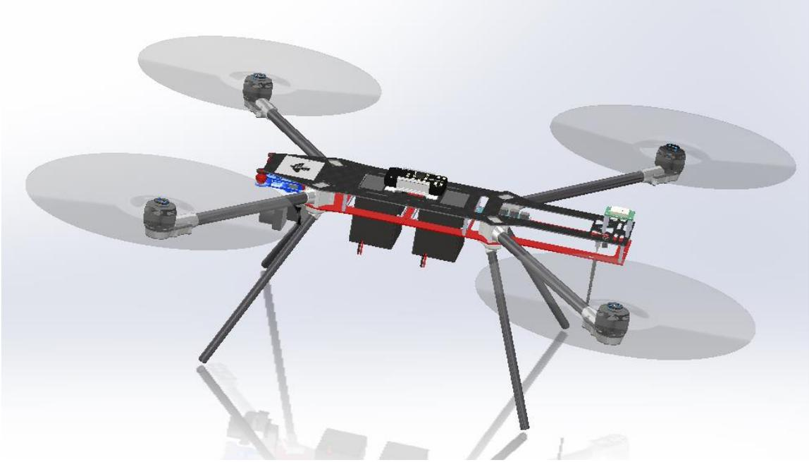
Figure 19. Condor Batteries Hung from the Upper Frame
