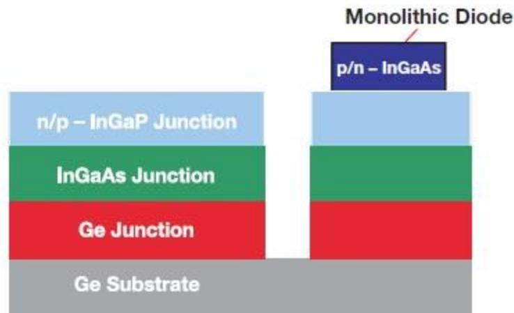
Figure 5. Molecular Makeup of an EMCORE BTJM Solar Cell.
