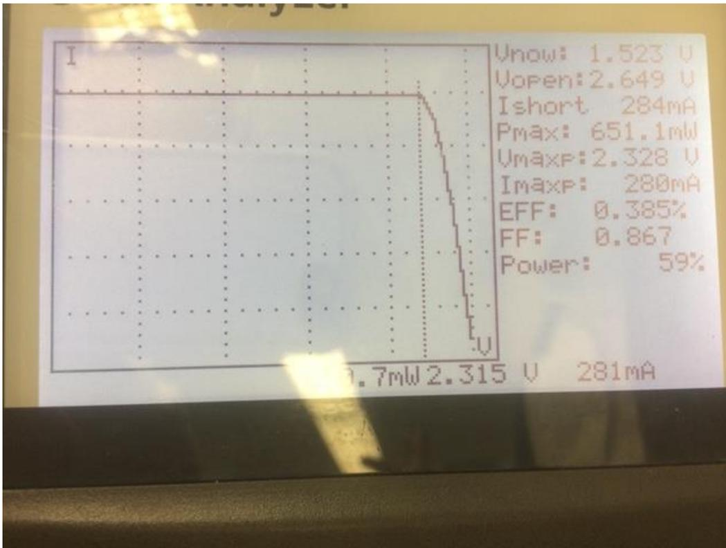
Figure 7. Solar Analyzer Analysis of a Single EMCORE BTJM 28% Solar Cell
