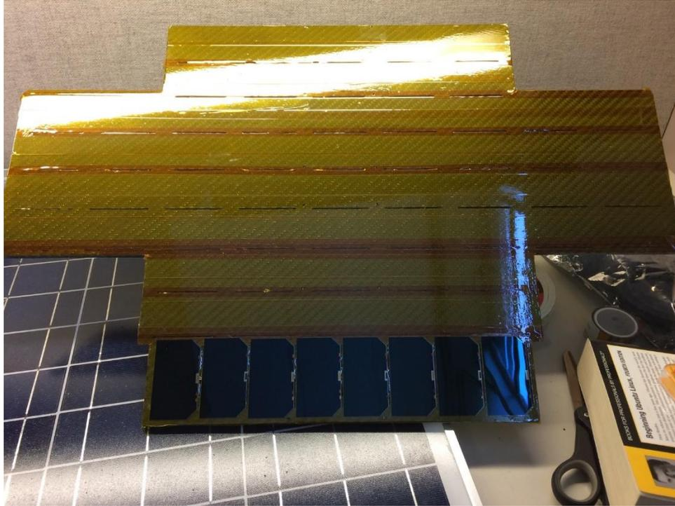
Figure 15. Insulating Kapton Tape Covering the Surface of Condor's PV Array
