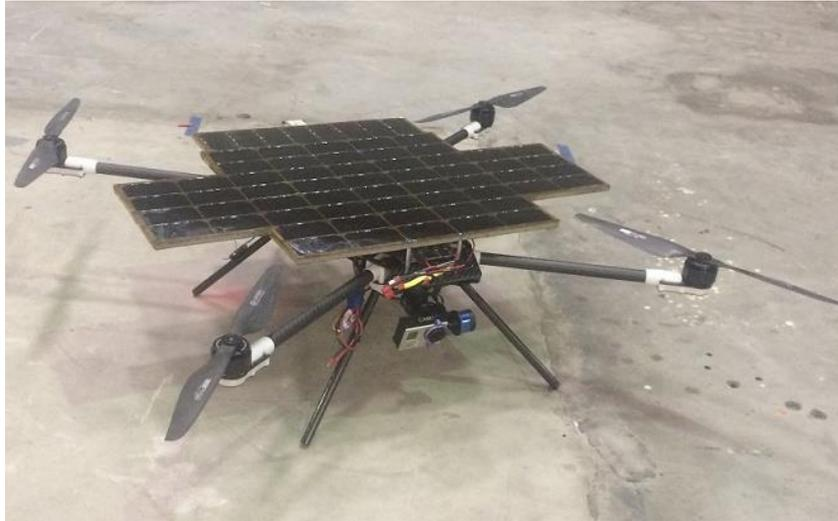
Figure 28. Condor Fully Assembled Indoor Flight Setup
