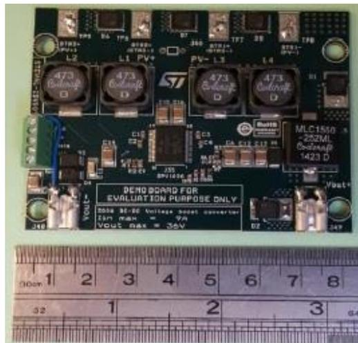
Figure 11. STMicroelectronics ISV009v1 MPPT as Manufactured. Source: [16].
