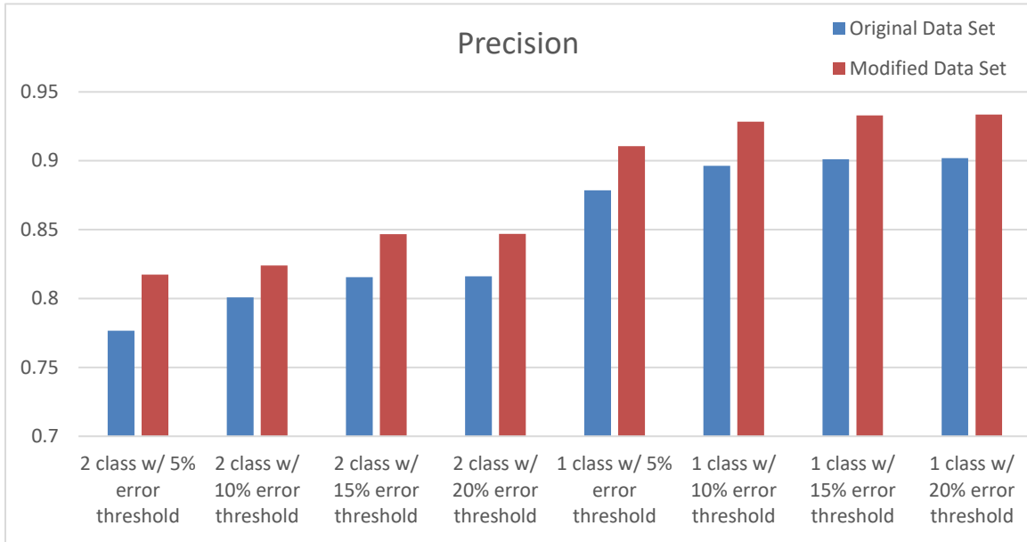
Figure 38. Comparison of Precision between two-classification and damage detection mode with original and modified data sets.
