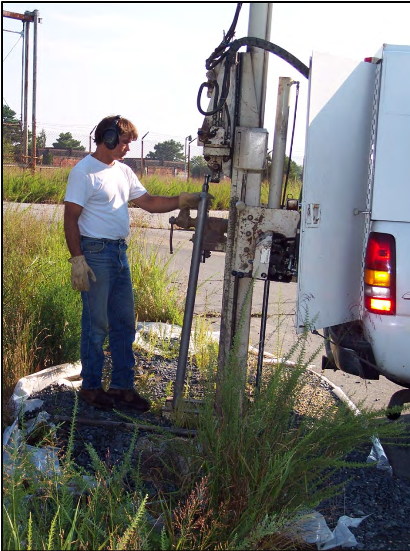
Figure C-19. Direct-Push Rig Sampling Location with Positive ^{241}\text{Am} Finding, Along Road Edge, South of Missile Area Entrance Gate.
