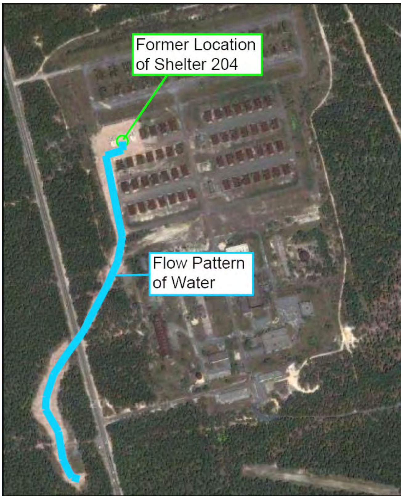
Figure A-10. General Flow Pattern of Water from Accident and Follow-on Storm Run-Off Surmised from Post-Accident Radiological Monitoring Activities.
