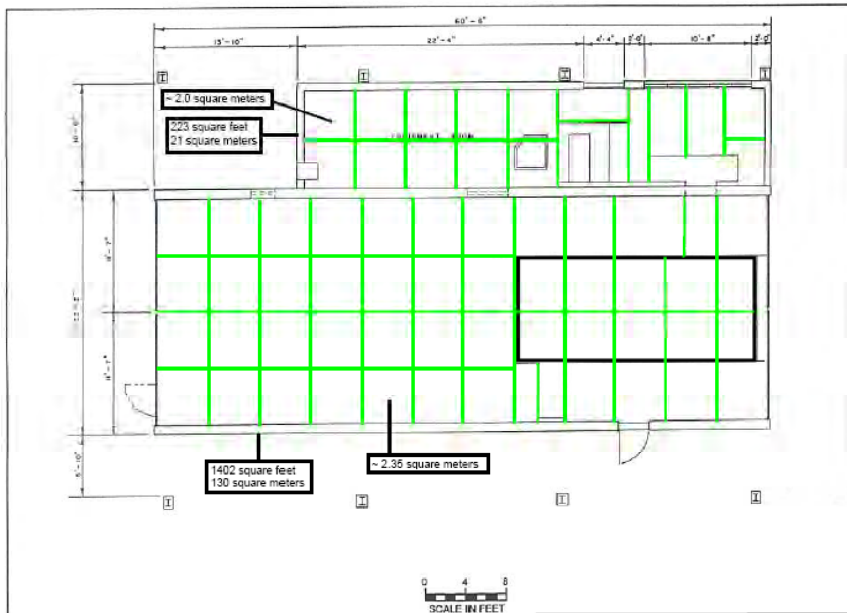
Figure D-2. Example Grid System for Shelter Floor and Pit Surveys.
