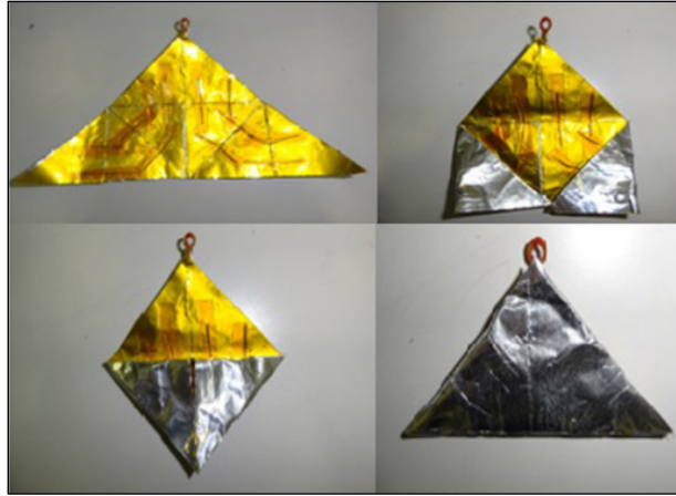
Figure 8. Opening Sequence of the Solar Sail Using SMAs. Source: [18].
