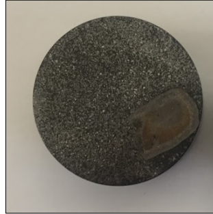
Figure 59. Prepared Sample Containing CNTs, Ni (5 \mu\text{m} ), Ti (45 \mu\text{m} ) and Gel Treated at 207 MPa for Characterization
