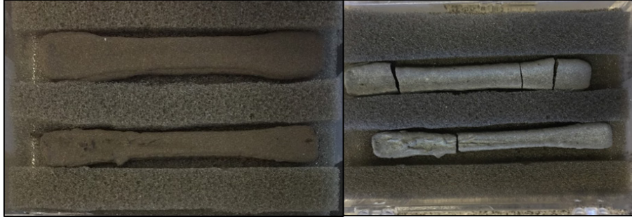
Figure 58. Samples Containing CNTs, Ni (5 \mu\text{m} ), Ti (45 \mu\text{m} ) and gel Prior to (left) and After HIPped at 207 MPa (right)
