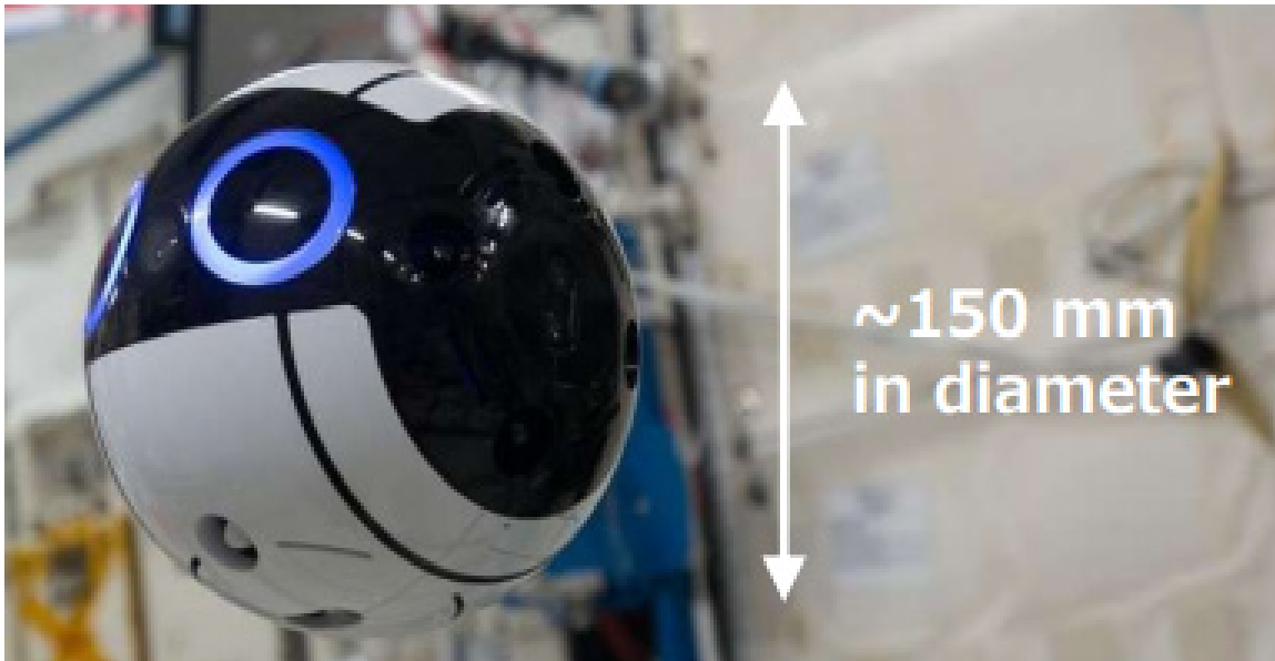
Figure 4. JAXA Int-Ball. Source: Japan Aerospace Exploration Agency (2017).
