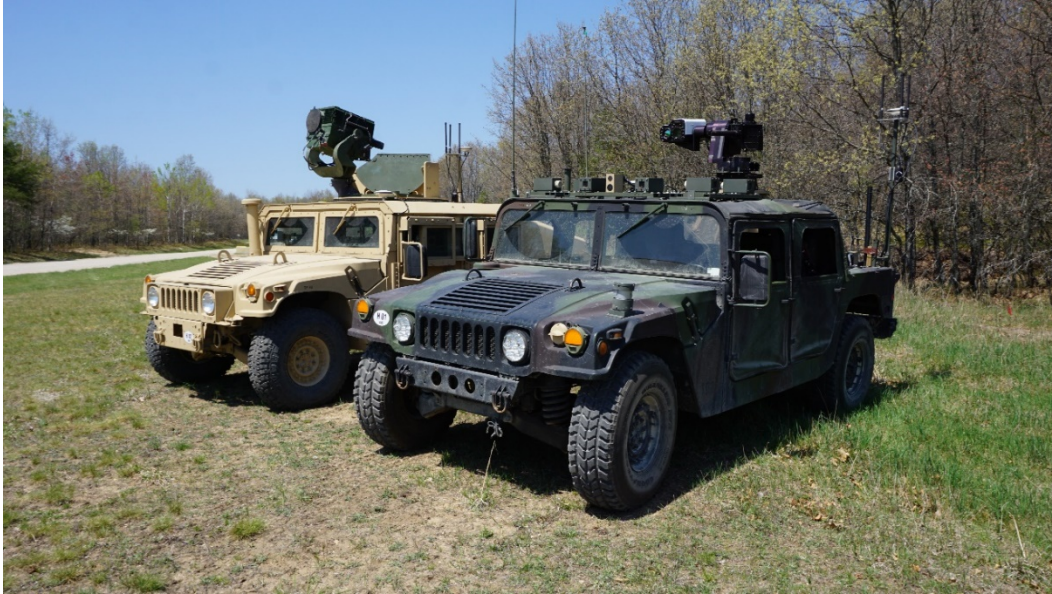
Fig. 1 Image of the real-world manned vehicle (left) and robotic weaponized vehicle (right)
