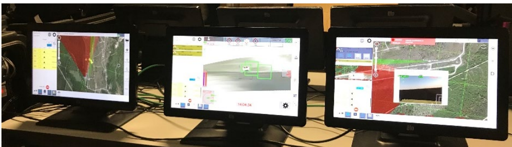
Fig. 2 Example of the three WMI displays for the commander (left), robotic vehicle gunner (center), and robotic vehicle operator (right)
