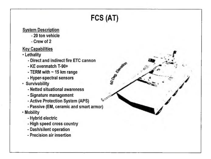
The FCS Anti-Tank variant is a 20-ton vehicle with a 2-man crew and a direct fire ETC weapon capable of beyond-line-of-sight fires with the Tank Extended Range Munition (TERM) round. The gun elevates up to 60 degrees to enable precision fires at elevated targets in urban environments with programmable levels of lethality.
