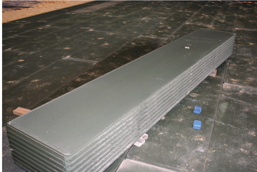
Figure 2.5. AM2 airfield mat stack.
