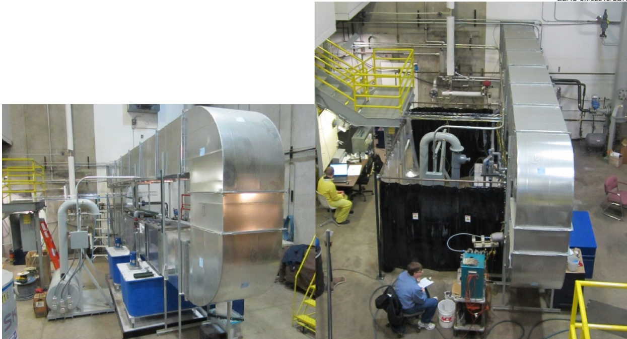
Figure 2. The EERC's dry cooling test facility after fabrication (left) and during an aerosol emission test (right).
