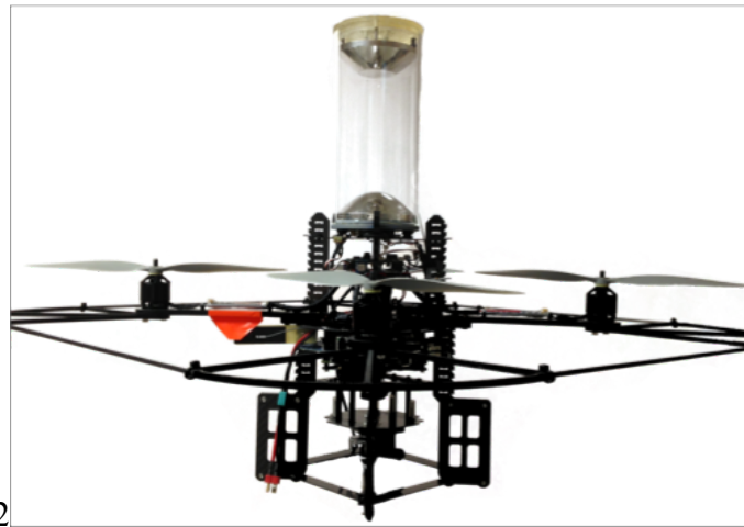
Fig. 1 Synthetic catadioptric single-camera omnistereo system, whose main tangible are components: 1.a-b) hyperboloid- planar combined mirror at top, 2) hyperboloidal mirror at bottom, 3) camera, 4) transparent cylindrical support, and 5.1-2) blue-red lips acting as circular markers during image processing. Fig. 2 The omnistereo vision prototype installed on the AscTec quadrotor MAV
