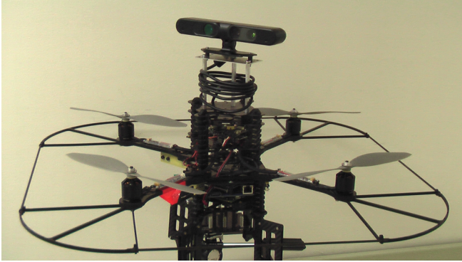
Fig. 10. The CityFlyer MAV equipped with an Asus Xtion Pro Live RGB-D
