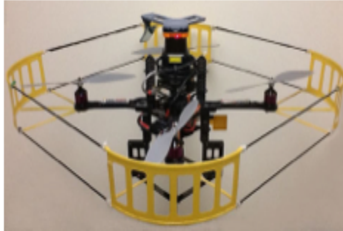
Fig. 7 The City-Flyer quadrotor MAV equipped with a Hokuyo laser scanner
