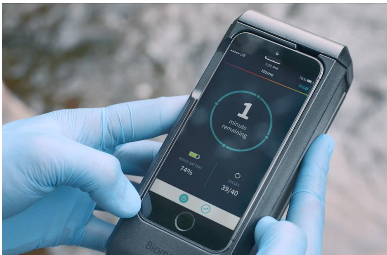
Figure 1. A Biomeme two3™ hand-held real-time PCR device along with the integrated iPhone (Biomeme, Inc., Philadelphia, PA)
