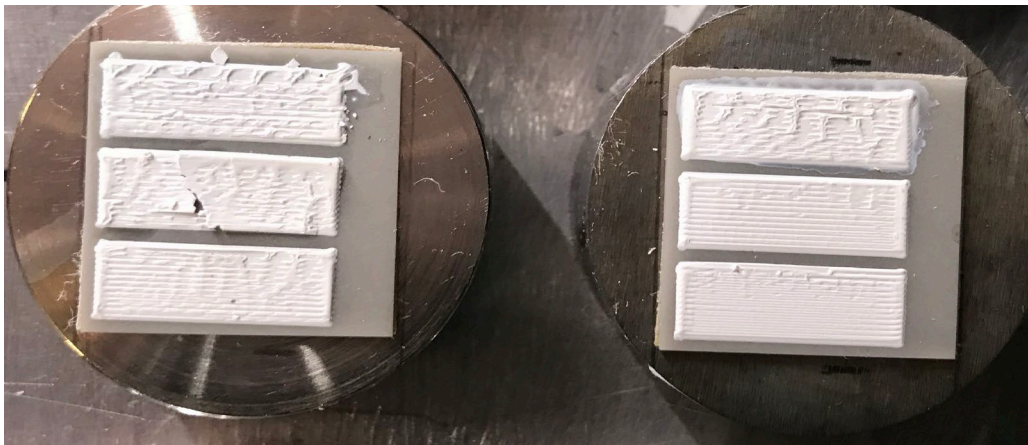
Fig. 12 Dispensed multilayer parts assembled with the ARL n-Script
