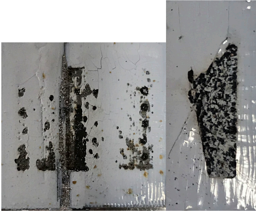
Fig. 32 Samples 3 (left) and 10 (right) were lased with higher laser energy. Sample 3 shows a combination of removal of slurry from the base and blackened slurry. Sample 10 shows blackened slurry.
