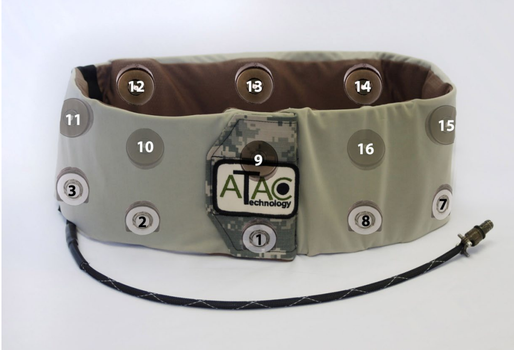
Fig. 5 Prototype dual row tactile belt. Each belt contained a row of eight C-3 factors (top) and a row of eight EMR factors (bottom). Factors 9 and 1 correspond to the front of the abdomen.
