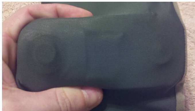
Fig. 6 Prototype dual row tactile belt (inside part touching the skin)
