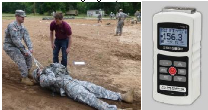
Figure 14. Field measurement of friction forces during a dummy drag test using a Mark-10 Series 5-strain gauge dynamometer.
