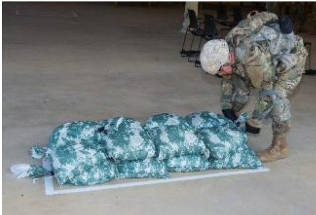
Figure 9. The final fighting position configuration was comprised of a stack of 16 sandbags weighing 45 lb. They were arranged in two layers of eight bags in a 2 long x 2 high x 4 wide layout.
