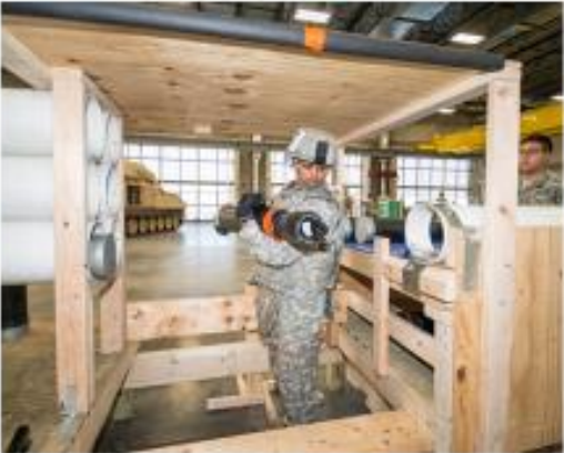
Figure 41. The load the main gun simulator in the final developmental format.
