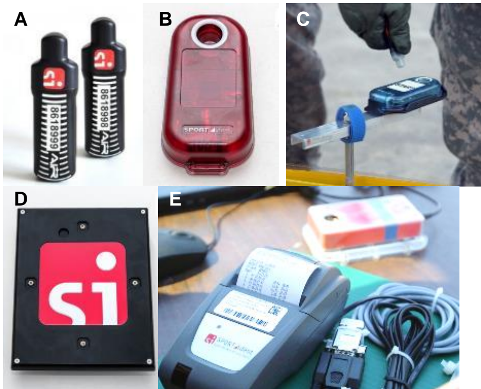
A. SPORTident Active Card (SIAC) RFID data stick; B. Start/ finish controls; C. Soldier placing stick into control; D. SIAC timing gate; and E. Download/printer station
