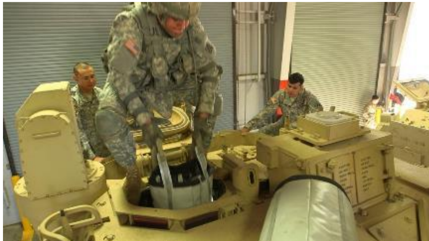
Figure 22. A Soldier pulling the lift bag from the hatch of a BFV.
