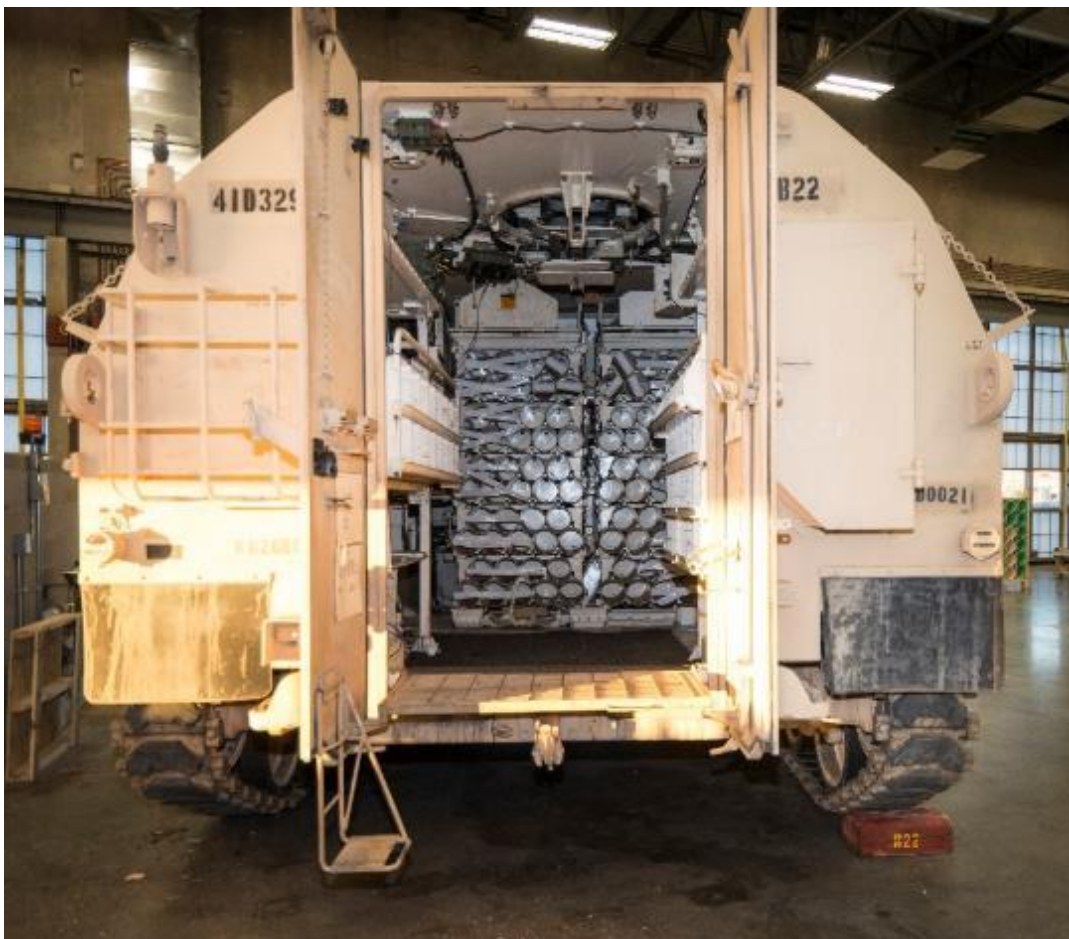
Figure 45. The open back door of the FAASV showing the ammunition racks at the front of the vehicle.
