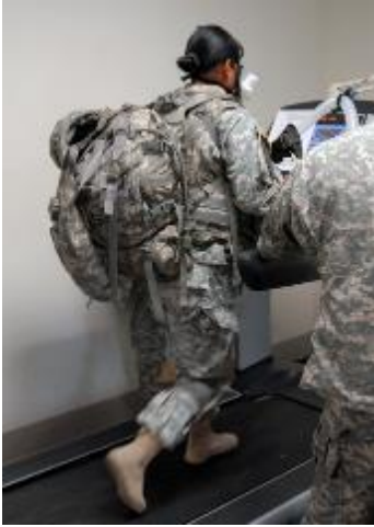
Figure 2. Open circuit spirometry measures on a Soldier performing simulated road march on a treadmill
