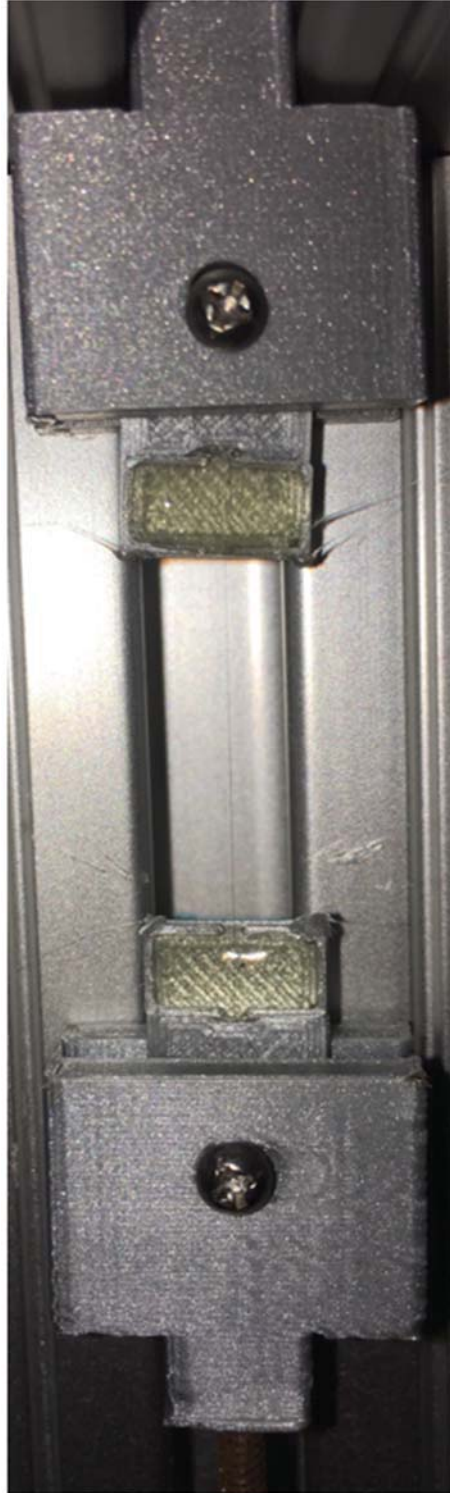
Figure 6: Fiber holder with connector arms melted away by soldering iron
