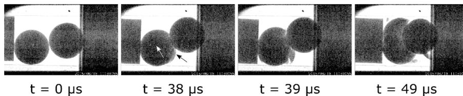
**Figure 7:** The high speed X-ray images for multi-particle compression. The cracking initiated near the contact points for soda lime glass particles and near the center for PMMA particles. The particles in glass particles spanned the contact points and ultimately particle with maximum particle-particle contacts fragmented explosively. For PMMA particles, the particle fractured in two hemispherical fragments.
