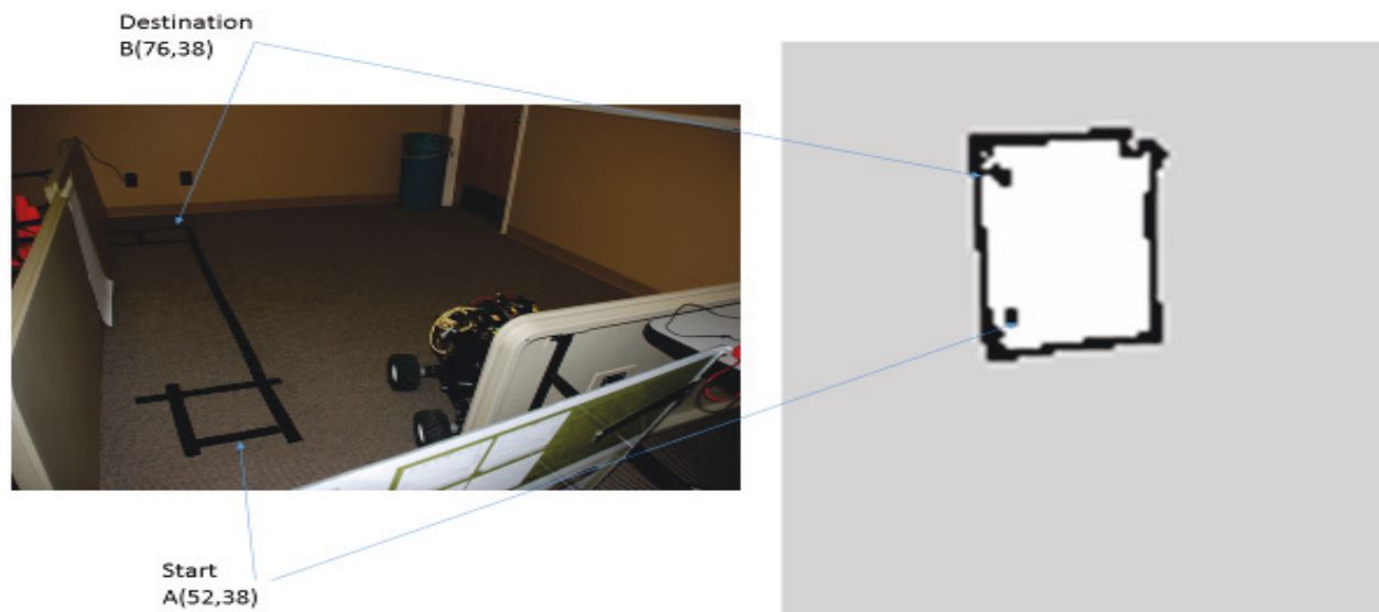
Figure 34. Test Site One without cones and the SLAM generated map.
