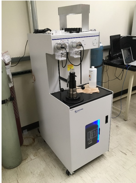
Figure 1. Micromeritics AutoPore V mercury porosimeter.
