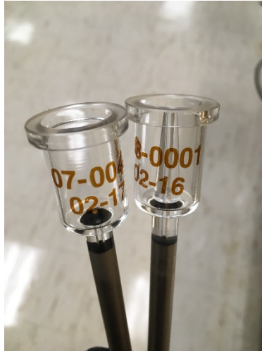
Figure 4. Penetrometers for mercury porosimetry. Left: suitable for larger samples. Right: suitable for powders.
