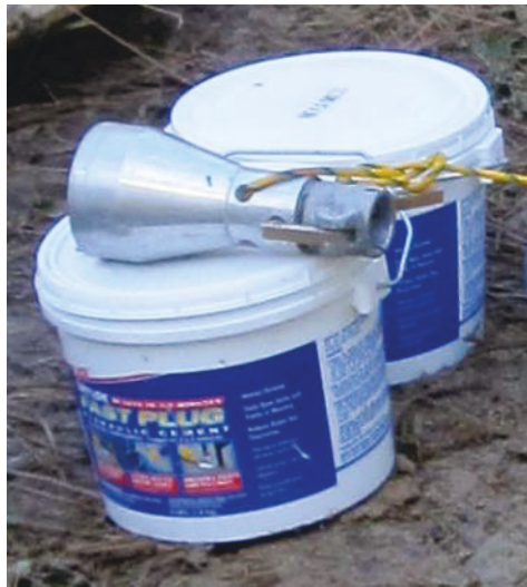
Figure 8. Installation magnetic cap with paracord.
