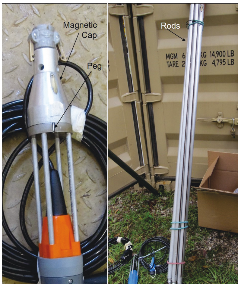
Figures 4. Installation hardware components are the magnetic cap (4A) and segmented rods (4B). Figure 4A shows a close-up view of the tight fit of the magnetic cap attached to the sensor plate with one peg visible to aid in controlled release of the cap.
