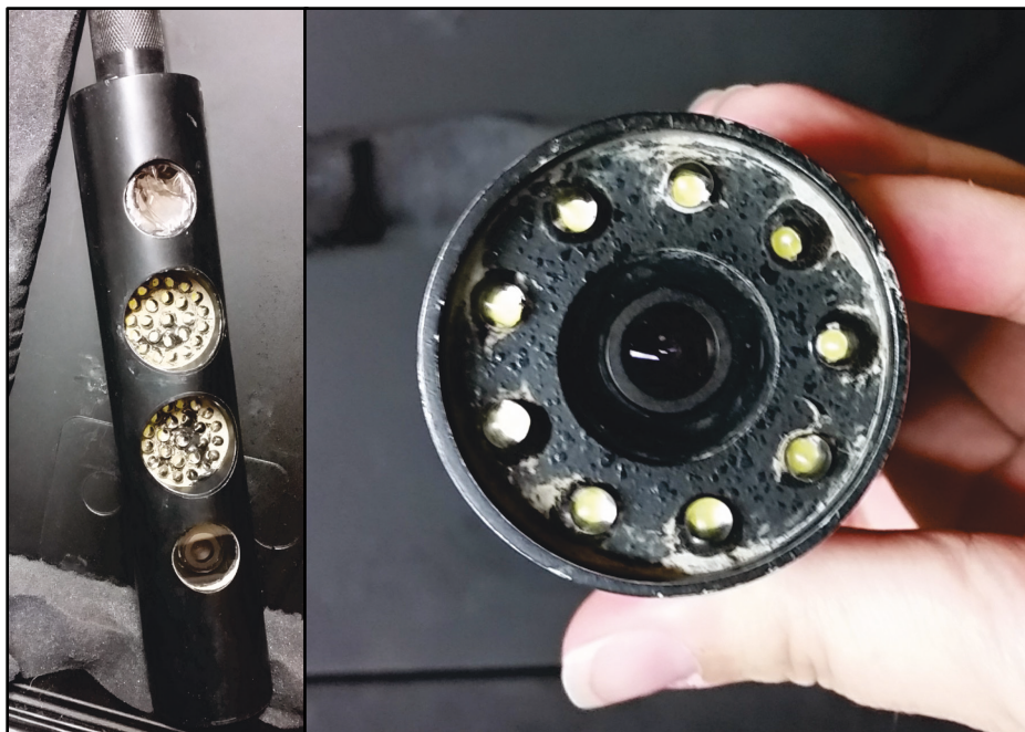
Figure 14. Borehole camera front and bottom view.
