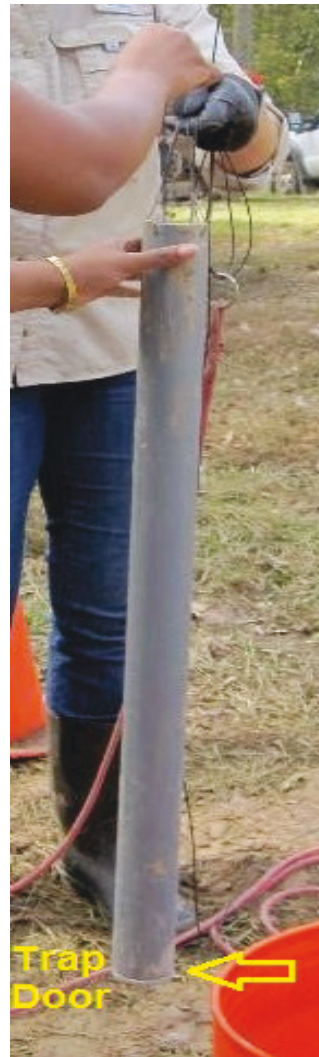
Figure 15. Using PVC pail with trapdoor to lower Drylok powder down to the sensor.
