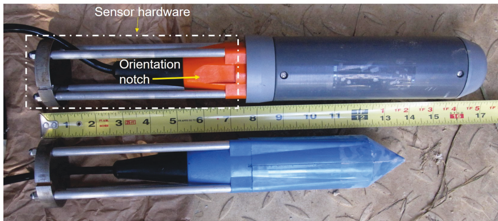
Figure 5. Three-component sensor hardware from prior experiment (bottom) and this experiment (top). The X or north direction for the sensor is shown by the notch in the orange part of the exterior casing.
