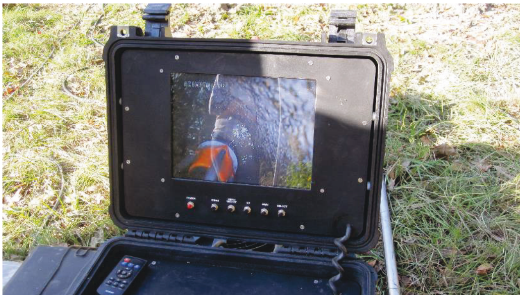
Figure 17. Screen shot from downhole camera to confirm sensor installation process.
