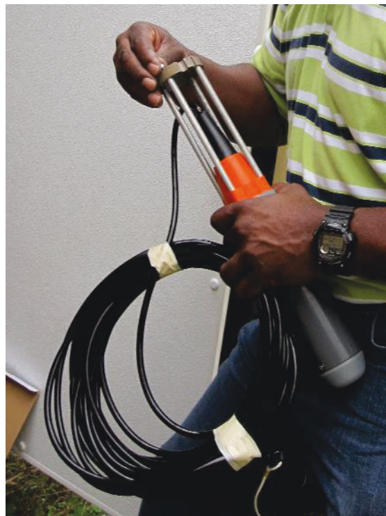
Figure 6. Installing sensor hardware plates and rods on three-component sensor.
