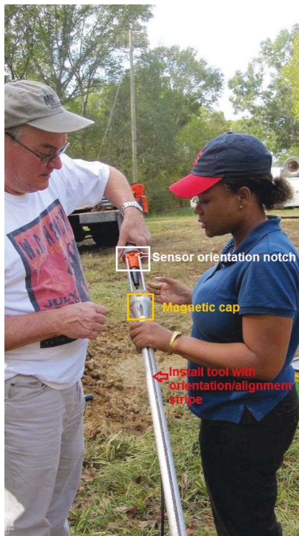
Figure 10. Sensor with orienting notch (orange part), magnetic installation cap, and install tool with orientation stripe.
