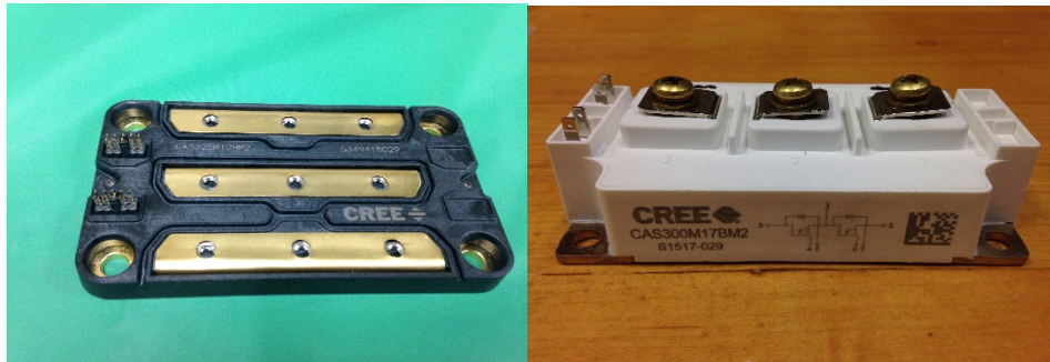
Fig. 4 A 1.2-kV, 3.7-m \Omega , 325-A module (left) and a 1.7-kV, 8.0-m \Omega , 300-A module (right)
