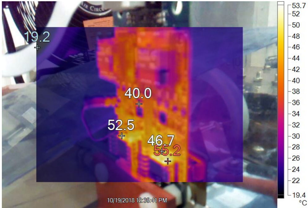
Fig. 23 Final temperature measurements of the front side of the driver board when V_{supply} was 600 V
