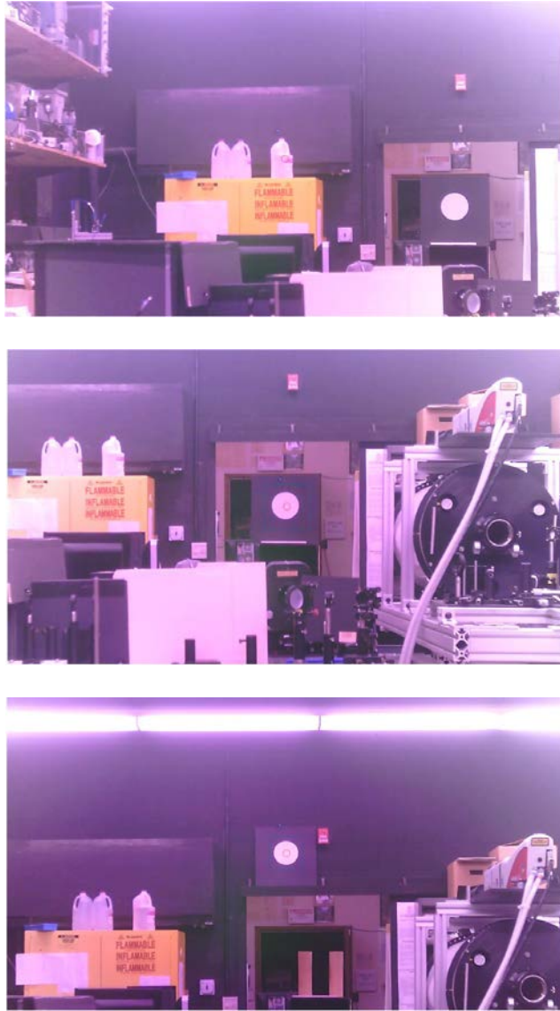
Figure 30. The top figure shows the image before the user has selected the target template region. The red circle in the center of the image is the position of the laser. The target is the white circle seen on the right of the image. After user defines the white circle as the target, the system automatically follows the target as shown in middle and bottom figures.
