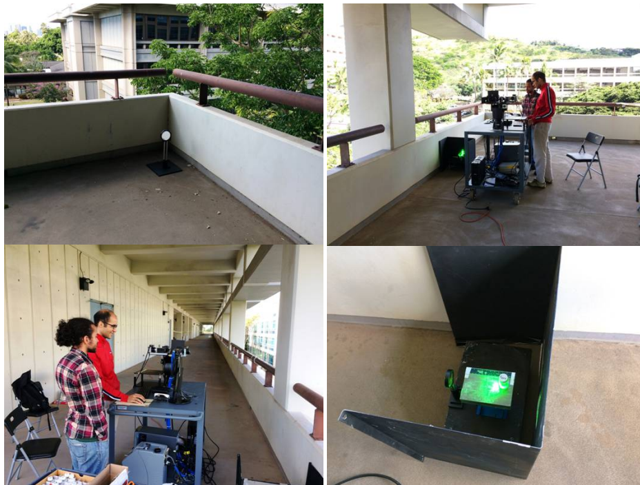
Figure 13. Field test at 246 m target distance. A 6" mirror (shown in top left image) was used at the end of the 128 m long hallway to reflect the laser back to excite the targets placed behind the system as shown in the images on the right.
