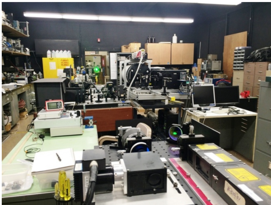
Figure 4. Lab setting for testing remote Raman system at 20 m target distance under bright condition. Targets are located on the far side of the room where green laser spot is visible.
