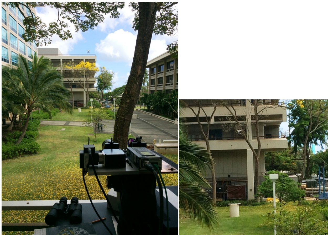
Figure 37. Outdoor testing of the system. For eye safety, the system was placed on the second floor and targets were placed on a white drum shown on the far end of the image. The line of sight was several feet above normal human height except near the target, where guards were placed to stop people to walk in the laser beam.
