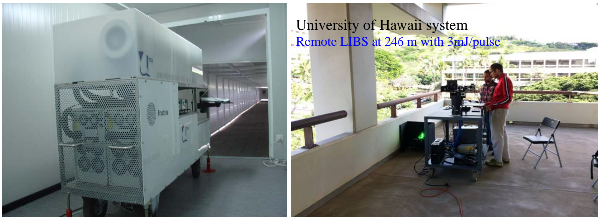
Figure 25. Comparison of the system size and detection range. On left is the remote LIBS system from Univ. of Malaga, Spain, with 50 m range using 1600 mJ/pulse laser energy at 1064 nm (Laserna et al., 2007). On the right is the ATR-FR method (Univ. of Hawaii) testing successful remote LIBS at 246 m with single laser pulse of 3 mJ/pulse (532 nm) and small collection optics.
