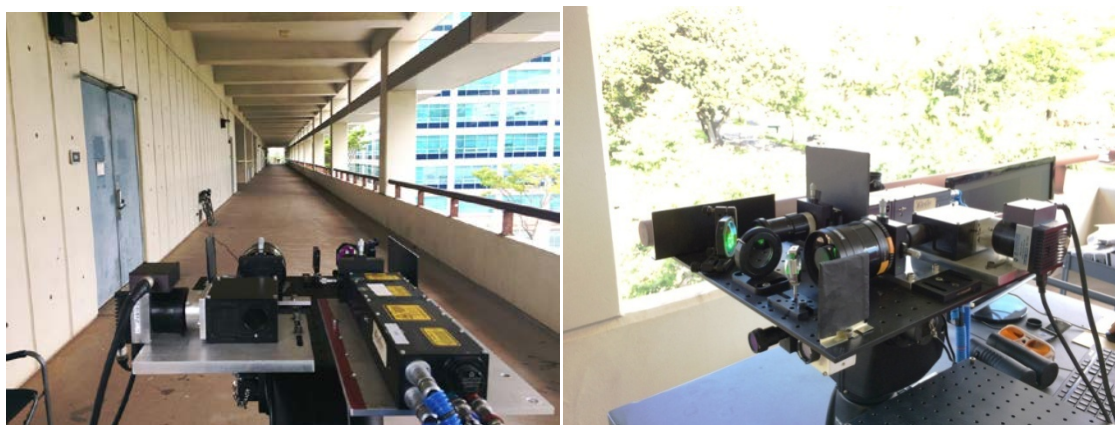
Figure 11. Compact remote Raman system with a 3" mirror lens as collection optics. Left image shows the field testing of the system with a target distance of 120 m during daylight. Right image shows close up image of the system.
