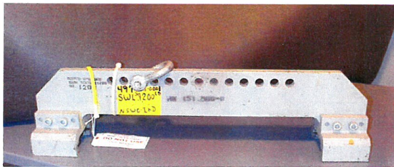
Picture 7 – Adapter, Missile Hoisting Mk 151 Mod 0
