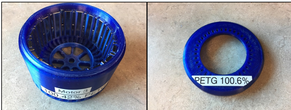
Figure 2 The Out-Runner Rotor: The Main Rotor Body with a Permanent Magnet Halbach Array and a Printed Screw-On Cap for Securing the Permanent Magnets
