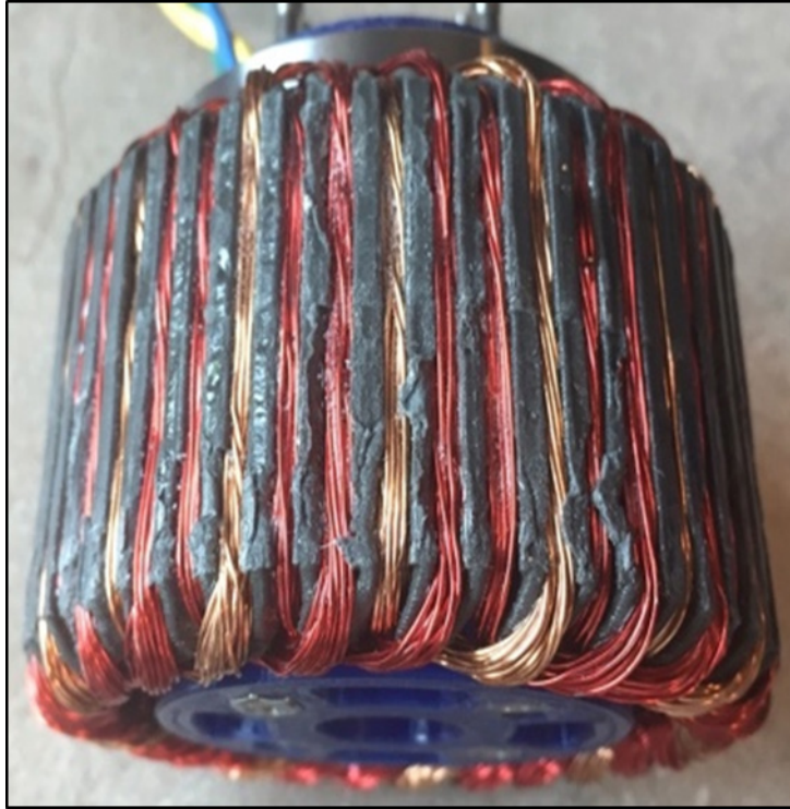
Figure 13 Stator Damage Due to Overheating
