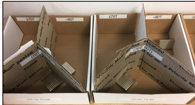
Figure 3 Binning System for Separating the Permanent Magnet by Weight and Magnetic Grade
