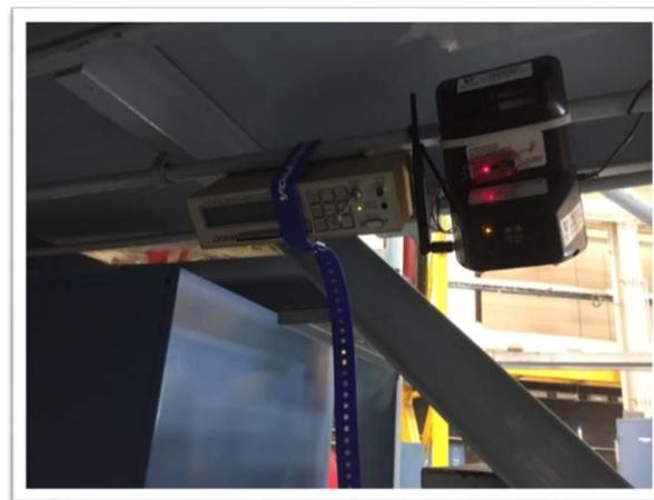
**Figure 3. USAF UMDS (right, black) and Grimm (left) affixed at approximately head height, ground level proximal to fighter aircraft (Hill AFB, UT Bldg 225).**
