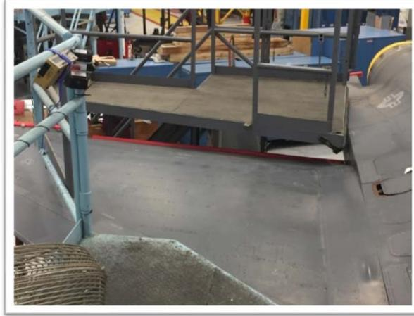
**Figure 4. USAF UMDS (right, black) and Grimm (left) affixed at approximately waist height, wing level proximal to fighter aircraft (Hill AFB, UT Bldg 225).**
