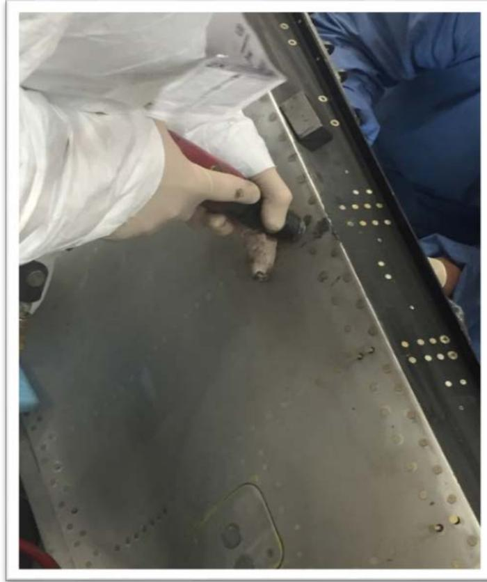
**Figure 26. Workers metal grinding while wearing proximity sensors (in pocket) and wearing personal noise dosimeter.**
